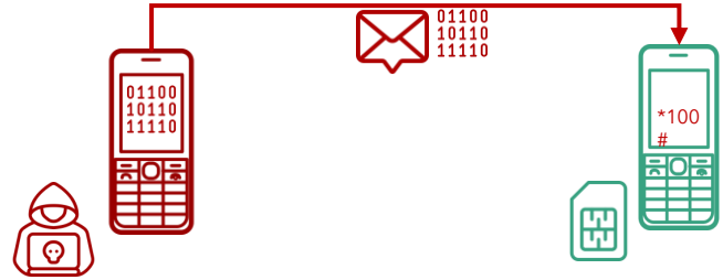
b. Testing susceptibility to binary OTA attacks (SIM jacker, WIB attacks)
