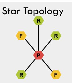
All devices communicate to PAN co-ordinator which uses mains power
