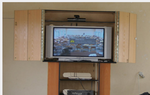
Figure 2.1: WoredaNet equipment, comprising, from top to bottom: a video camera, a plasma TV screen, a decoder and an amplifier/equalizer
