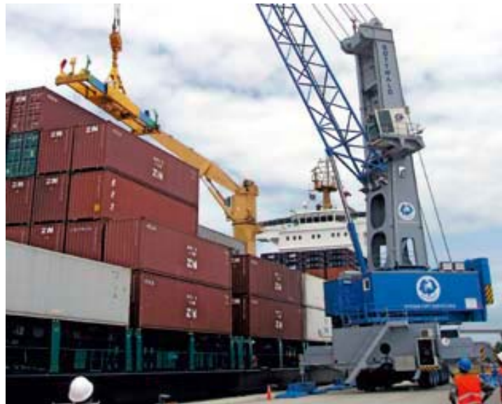
Picture 2: Gottwald HMK 260E Mobile Harbor Crane in Port of Paramaribo
