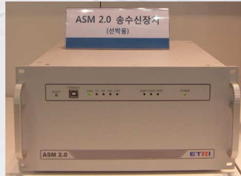
RF Transmitter Module for ASM Coast/Ship station
