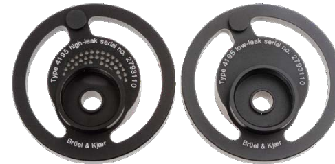
type 3.2 Simplified pinna simulator. (high/low leak)
