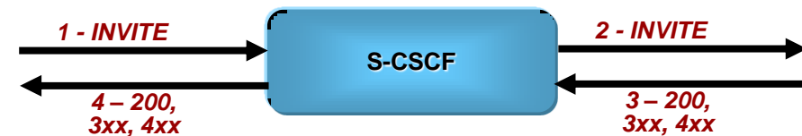
Model 5: A SIP leg is passed through the S-CSCF without Application Server involvement
