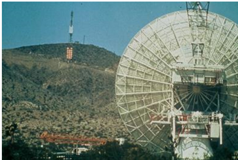
Figure 29: One mile point-to-point power transmission experiment with a 26 m parabolic antenna and a 450 kW, 2.388 GHz klystron as a transmitter and a 3.4 \times 7.2 m rectenna array as a receiver
