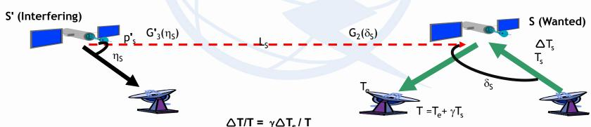
$\triangle T/T = 10\log \gamma + 10\log(p'_s) + G'_3(\eta_s) - L_s + G_2(\delta_s) - K - T(dB)$
