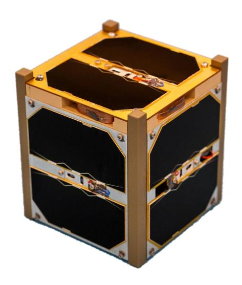
A "standard 1U" CubeSat has a volume of one liter - 10 cm cube and a mass of 1 kg, orbiting at 300-600 km circular orbit, 1W transmitter on 145 or 435 MHz amateursatellite service band. It's used for academic education, research and technology validation applications but also for complex science and governmental use.
