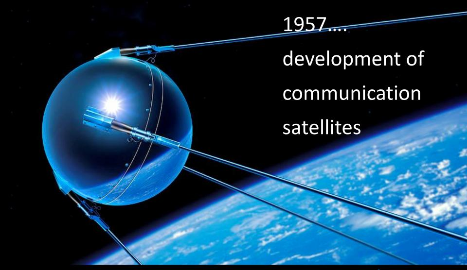
Sputnik 1 was the first artificial Earth "SMALL" satellite launched on 4<sup>th</sup> October 1957 with external radio antennas to broadcast radio pulses. It was a 58 cm diameter, 83 kg polished metal sphere with a 1 W transmitter on 20.005 and 40.002 MHz.
