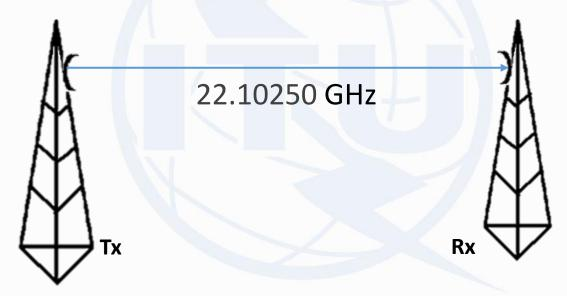
A point to point **micro wave link** in the **fixed service**:
