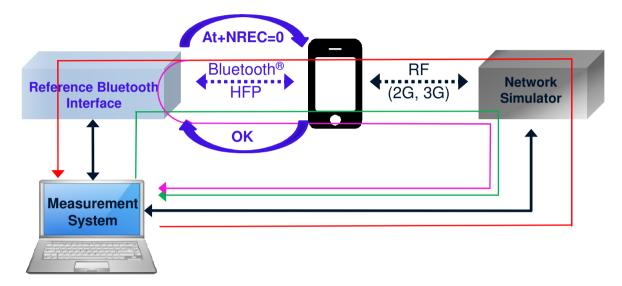
Testing of the phone in isolation in a simulated connection (HFP) to car HFT
