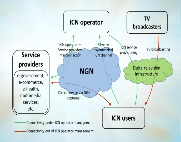
The process of service provisioning in ICN in typical deployment with NGN
