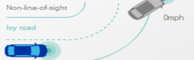
Blind curve hazard warning
