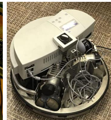
Photos of the implementation: SCW QKD system module, the gamepad issuing movement commands, the mobile robot with a camera operating through a QKD-protected channel.
