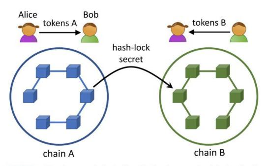
**FIGURE 1.** Atomic cross-chain trading. Having the same hash-lock value in the transactions on the two chains can ensure that either both of the two transactions (Alice and Bob exchanging tokens on the two blockchains) occur, once the hash-lock secret is revealed, or neither occurs.
