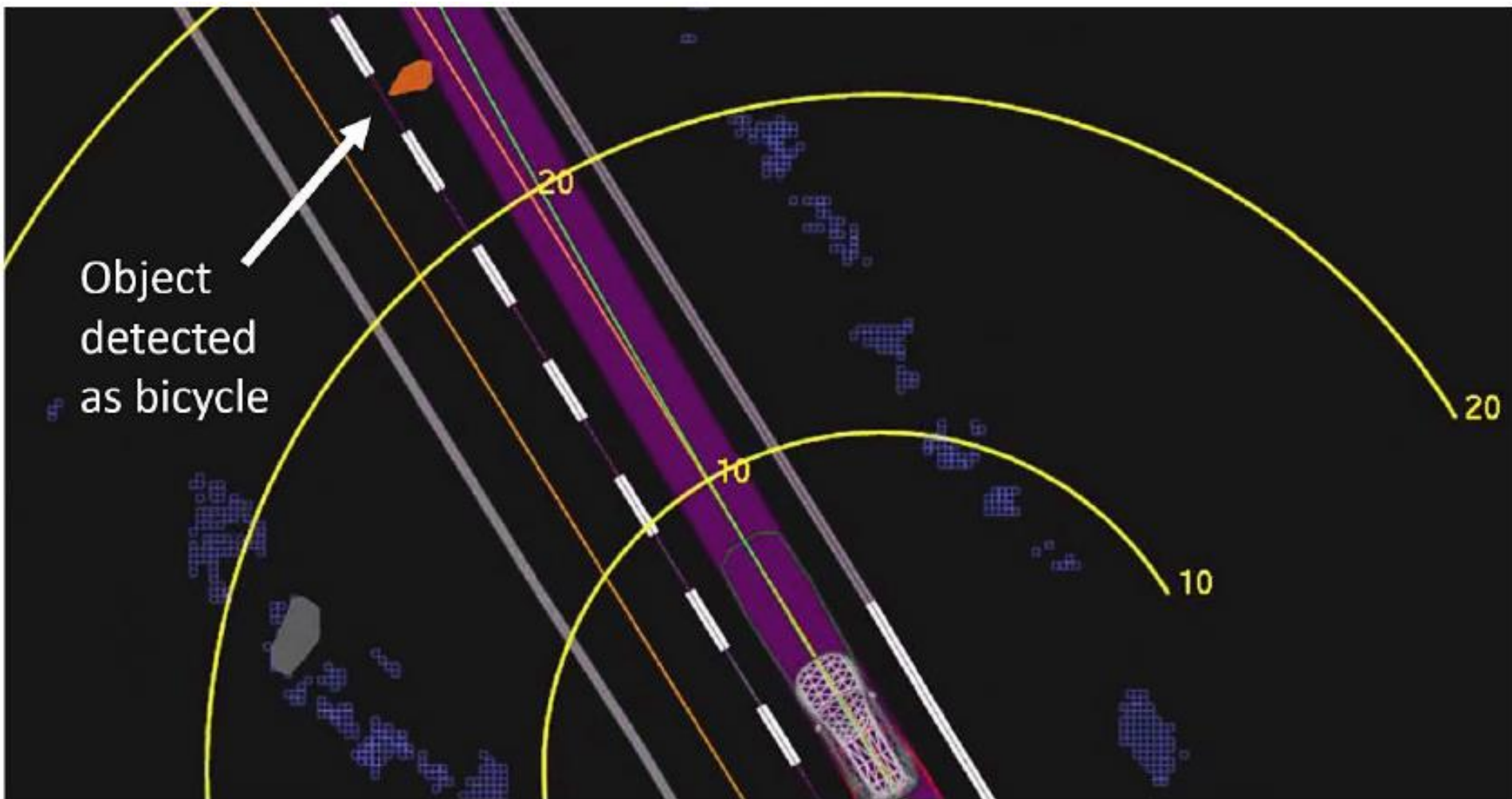
Figure 2. View of the self-driving system data playback at about 1.3 seconds before impact, when the system determined an emergency braking maneuver would be needed to mitigate a collision. Yellow bands are shown in meters ahead. Orange lines show the center of mapped travel lanes. The purple shaded area shows the path the vehicle traveled, with the green line showing the center of that path.
