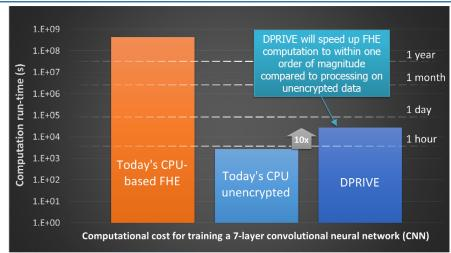
Program Objective: Design and implement a hardware accelerator to reduce computational run time for FHE to make it comparable to similar unencrypted data operations (within 10x)
