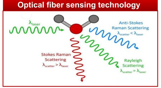
Optical fiber sensing technology can detect p anomalies and events by analyzing the characteristics of reflected and back-scattered optical signals, such as optical signal intensity, wavelength/frequency, phase, polarization, and so on.
