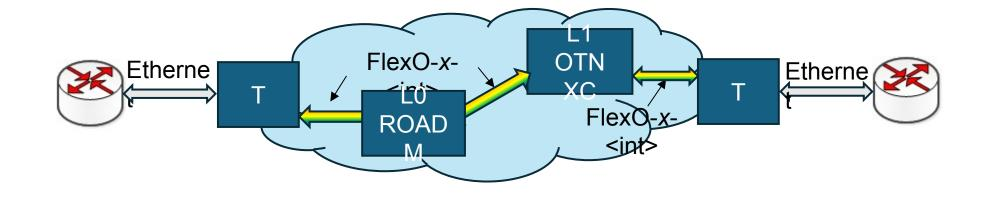
Direct router interconnect using Ethernet-optimized FlexO-*x*e
