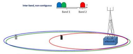
Primary Serving Cell (PSC), Primary Component Carrier (PCC), RRC connection and data Secondary Serving Cell (SSC), Secondary Component Carrier (SCC), user data Secondary Serving Cell (SSC), Secondary Component Carrier (SCC), user data
