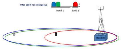
Primary Serving Cell (PSC), Primary Component Carrier (PCC), RRC connection and data Secondary Serving Cell (SSC), Secondary Component Carrier (SCC), user data Secondary Serving Cell (SSC), Secondary Component Carrier (SCC), user data To understand CA, 3GPP definitions must be understood:
