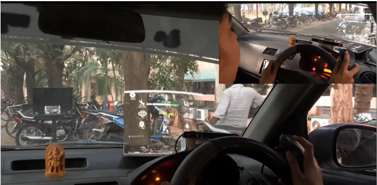
Figure 10: example of interactive eye gaze controlled HUD
