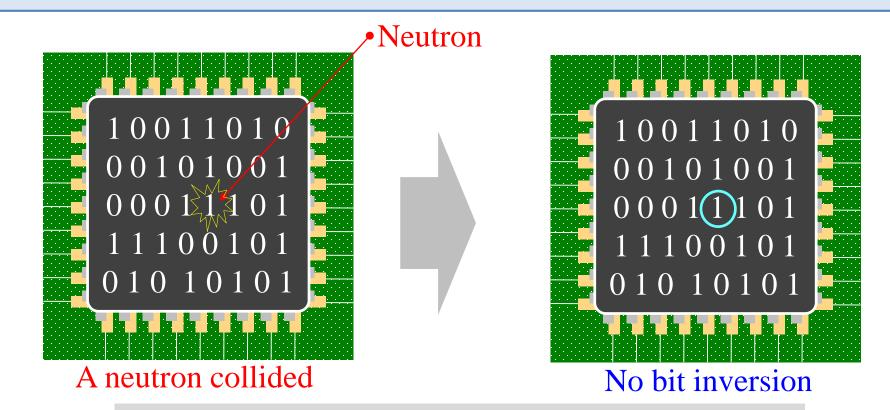
Ex1. Change in materialsEx2. Work on physical structureEx3. Reduction in areas where soft error occur
