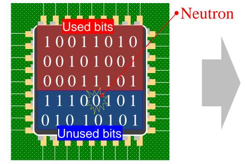
A neutron collided with unused bit 01010101 Unused bits Bit inversion occurred
