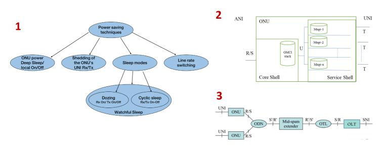
ITU-T G Suppl. 45 describes the power saving capabilities offered by the optical access context applied to its constitutive active devices' configurations: OLT, ONU and reach extenders. For each of them power saving concepts are listed across the diversity of ITU-T technologies: PON (ITU-T G.984, ITU-T G.987, ITU-T G.9807 & ITU-T G.9804), point to point (ITU-T G.9806) and multi-channel (ITU-T G.989).
