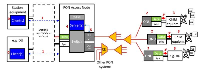
ITU-T G Suppl. 71 describes how CO DBA relates to the interaction between one or multiple protocol **Clients** [0] in station equipment and the protocol **Server(s)** [4] in the OLT, with exchange of **signalling messages** [1].
