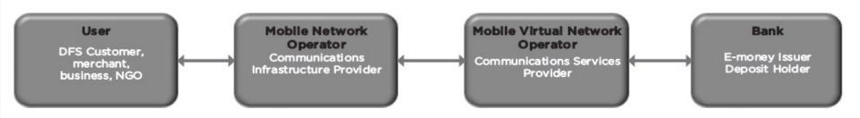
MVNO provides telecommunication services using MNO infrastructure, DFS provided with a bank or independently
