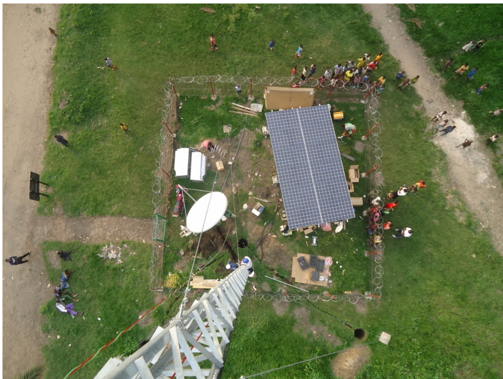
Figure 1: Aerial view of a base station backhauled by satellite powered by solar energy in Congo. Credit: Rascomstar
