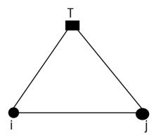
There are 2 exchanges, i and j, on the lowest level of an assumed hierarchical network structure, and another exchange, T, called the transit or tandem exchange, on a higher level.
