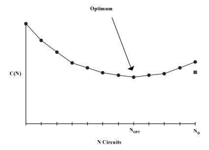
The points marked  $\bullet$  correspond to the above optimisation equation, valid for  $N = 0,1,2,...,N_D$ , and the point marked correponds to the cost for providing a direct route without overflow.
