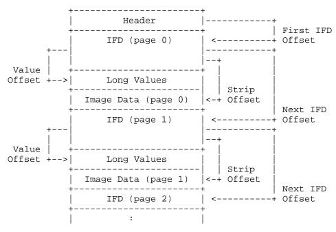
Using this file structure may reduce the memory requirements in implementations. It is also provides some support for streaming, in which a file can be processed as it is received and before the entire file is received.
