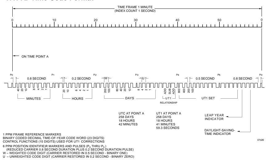
Fig. 3: Chart of Time Code Transmissions from WWVB
