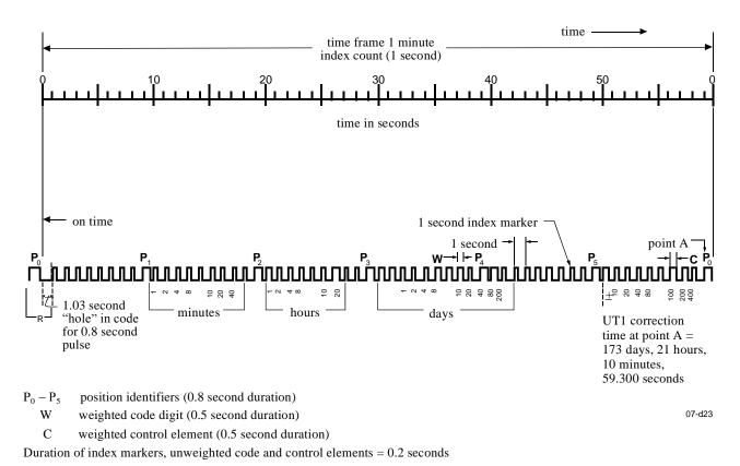
Fig. 2: Chart of Time Code transmissions from WWV and WWVH
