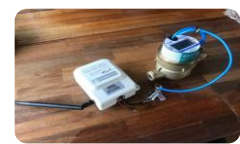
Water remote metering System for the elderly living alone
