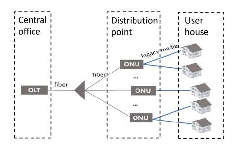
ITU-T Recommendations G.9700 and G.9701 for G.fast specify fibre to the distribution point (FTTdp) application by using 1G DSL links to connect user houses
