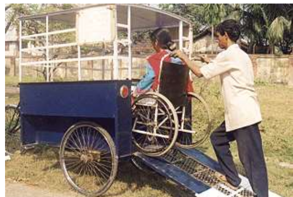
Figure 61: Accessible bicycle rickshaw. Photo: Access Exchange International
