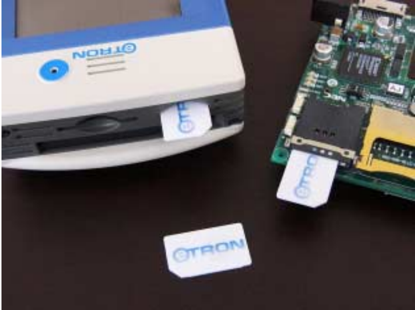
Photo. 2: eTRON Chip (SIM type)
