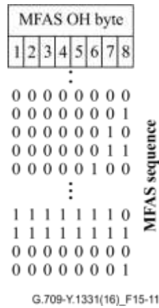
Figure 15-11 – Multiframe alignment signal overhead
