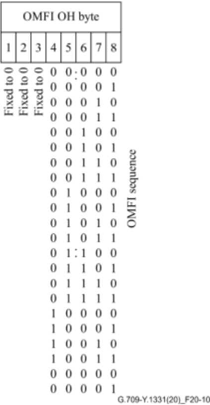
Figure 20-10 – OPUC n multiframe identifier (OMFI) overhead
