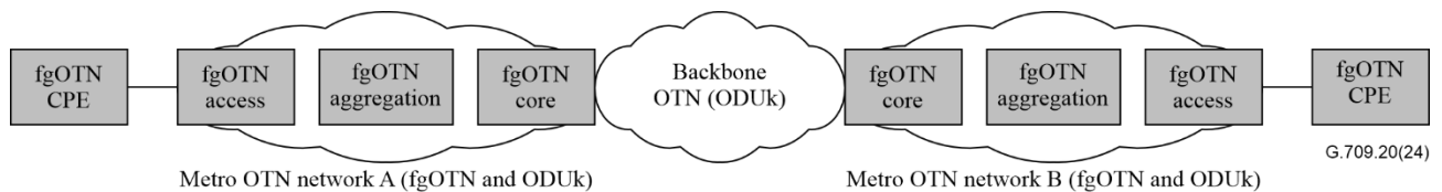
Figure A.1 – A reference network model for multi-domain fgOTN application
