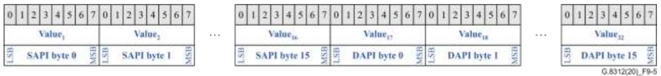
Figure 9-5 – TTI field of a CV message
