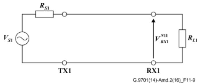
**Figure 11-9 – Voltage across the load without access cabling**
