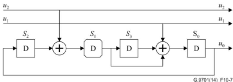
Figure 10-7 – Convolutional encoder: Finite state machine representation
