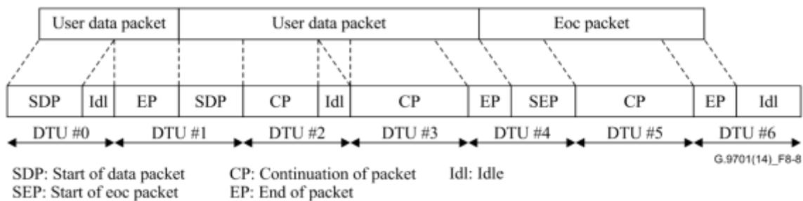
**Figure 8-8 – Example of mapping of packets for transmission in DTUs**
