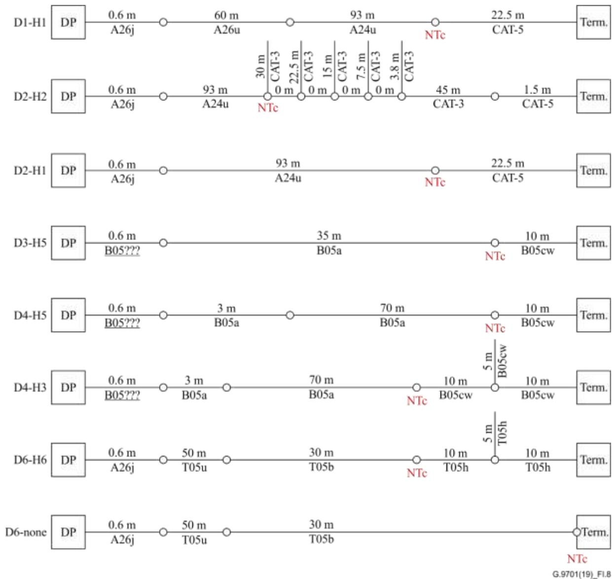
**Figure I.8 – Illustration of the reference combinations**
