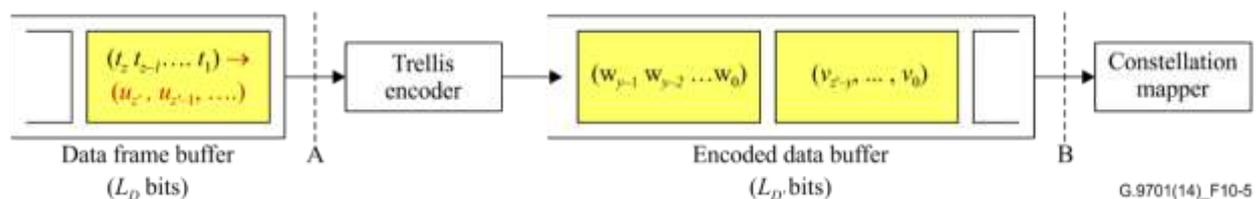
Figure 10-5 – Bit conversion by trellis encoder
