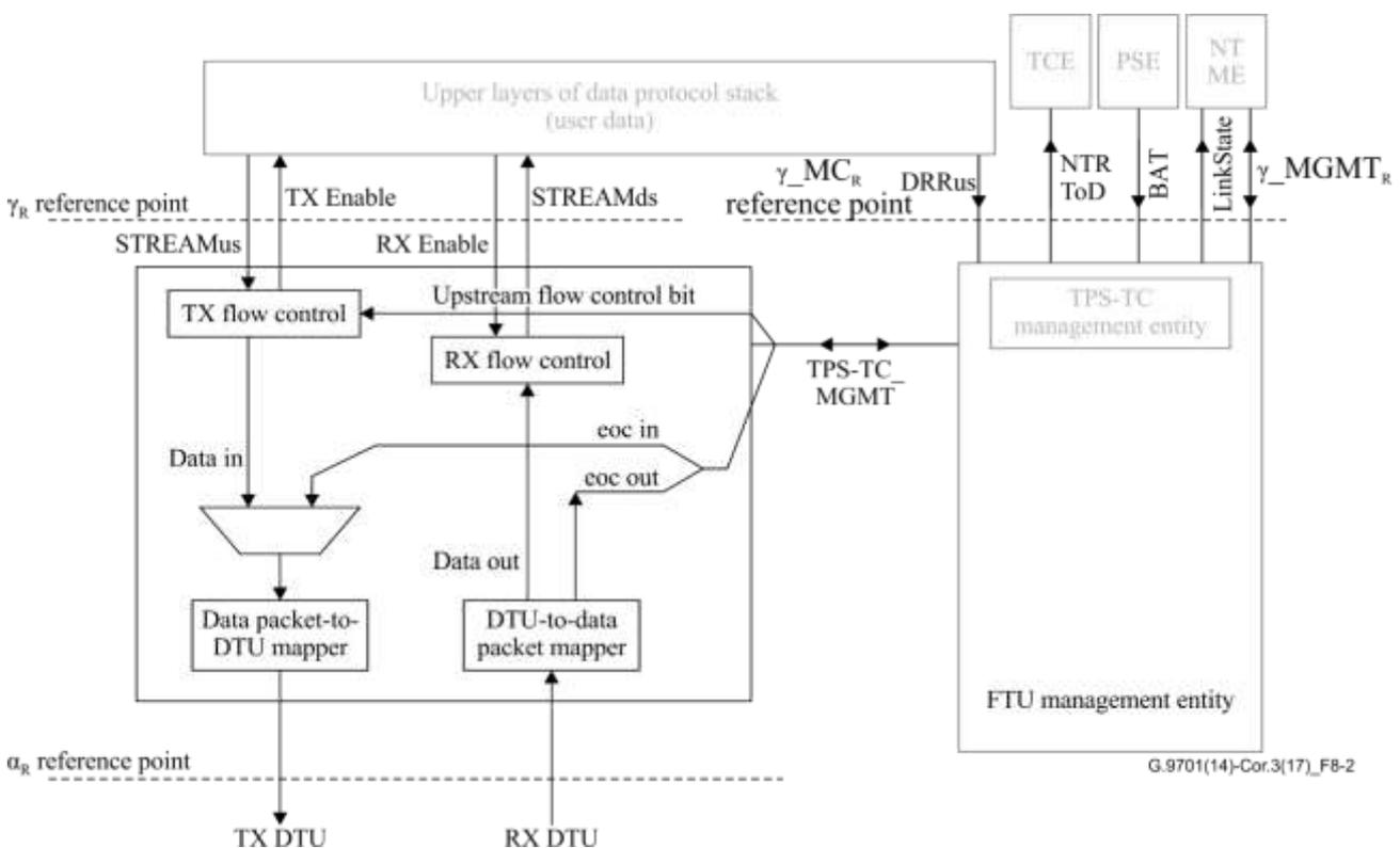
**Figure 8-2 – Functional reference model of the TPS-TC (FTU-R)**
