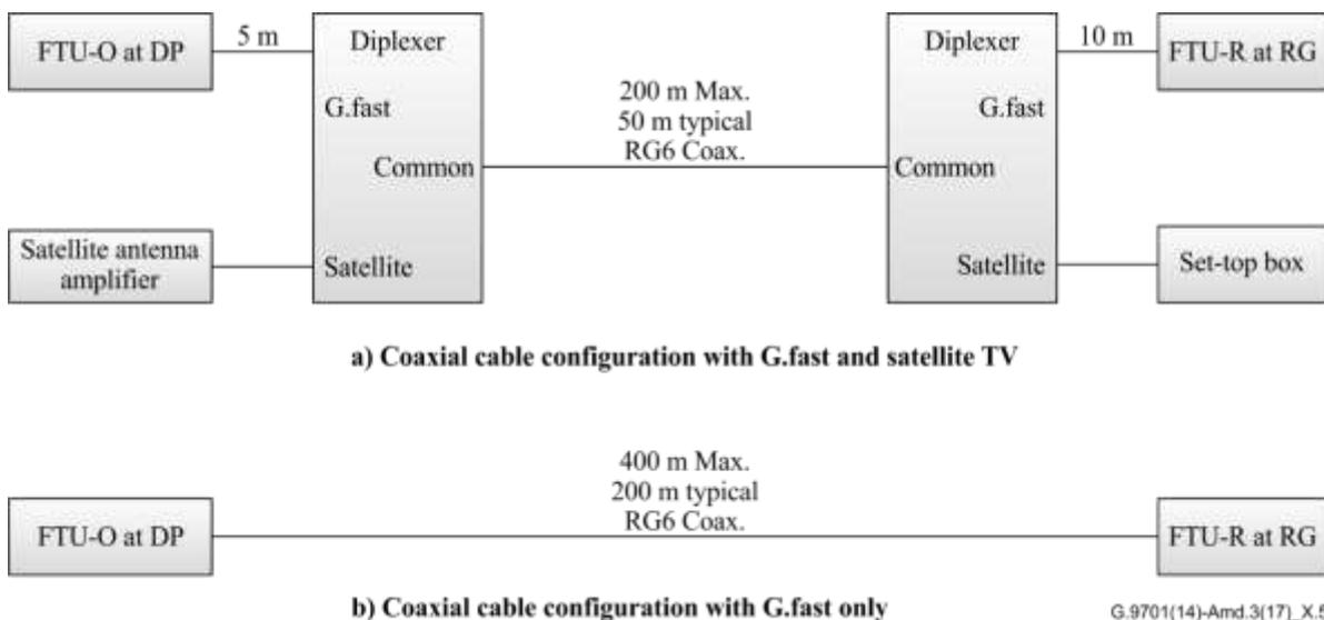
Figure X.5 – Coaxial cable configurations for two North American use cases:
