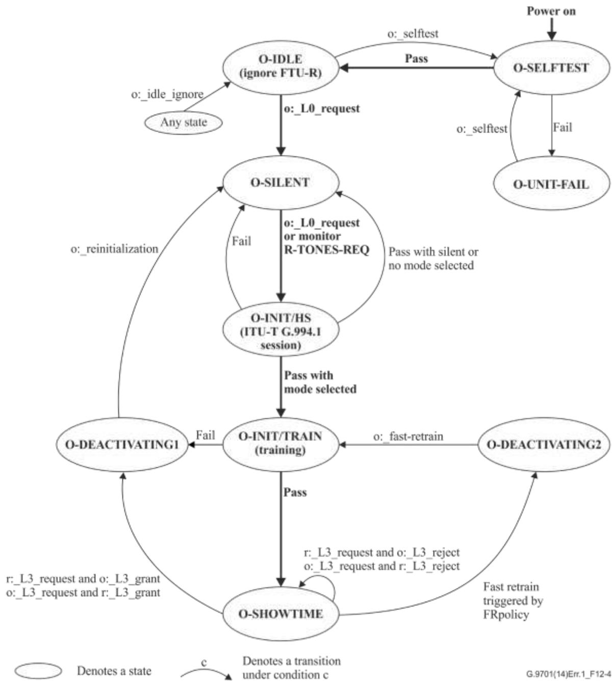
Figure 12-4 – State diagram for the FTU-O
