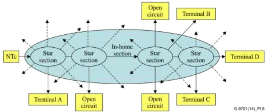
Figure I.6 – Overview of the in-premises wiring
