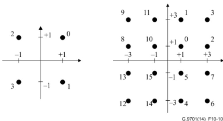
**Figure 10-10 – Constellation labels for  $b = 2$  and  $b = 4$**
