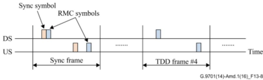
**Figure 13-8 – Example L2.1 transmission format for  $N=2$ ,  $M_{SF} = 8$**
