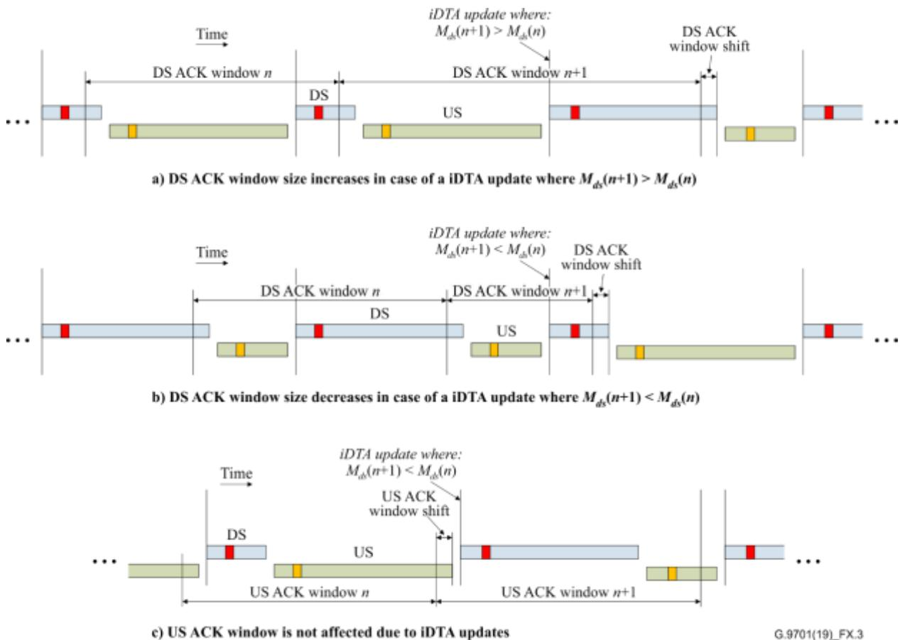
**Figure X.3 – Examples to illustrate the impact of an iDTA update on the ACK window size**
