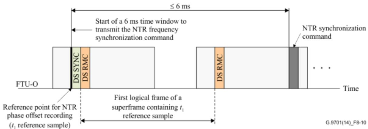
**Figure 8-10 – NTR offset recording and communication timeline**
