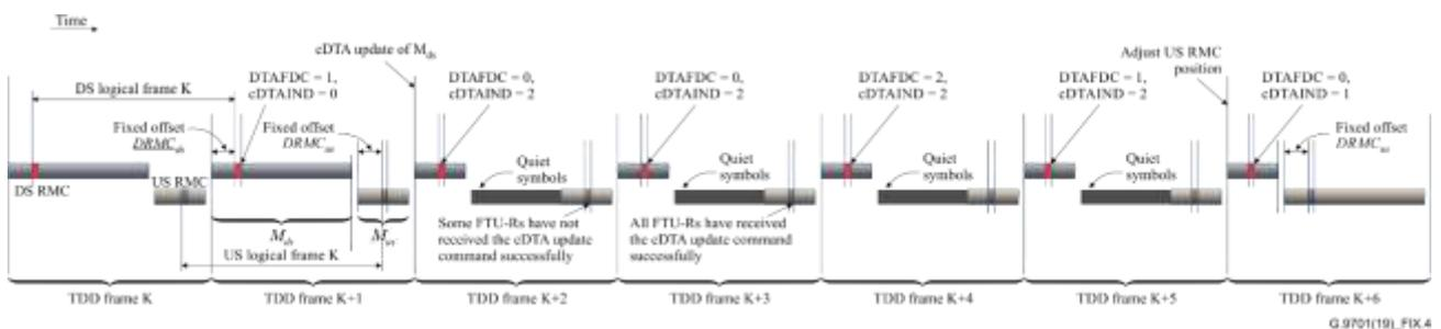
Figure IX.4 – Two-step cDTA procedure using upstream quiet symbols
