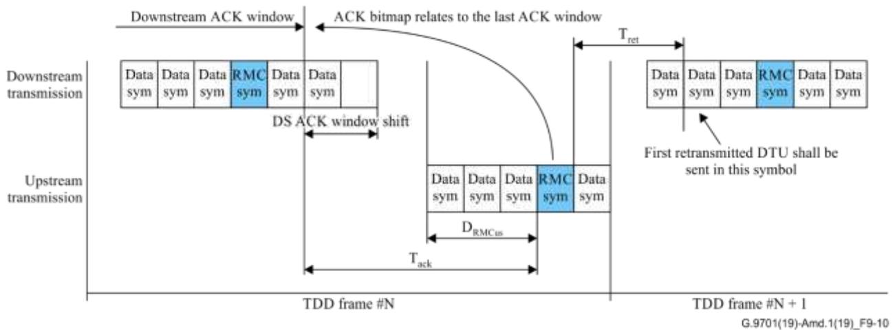
**Figure 9-10 – Illustration of parameters  $T_{ack}$  and  $T_{ret}$**
