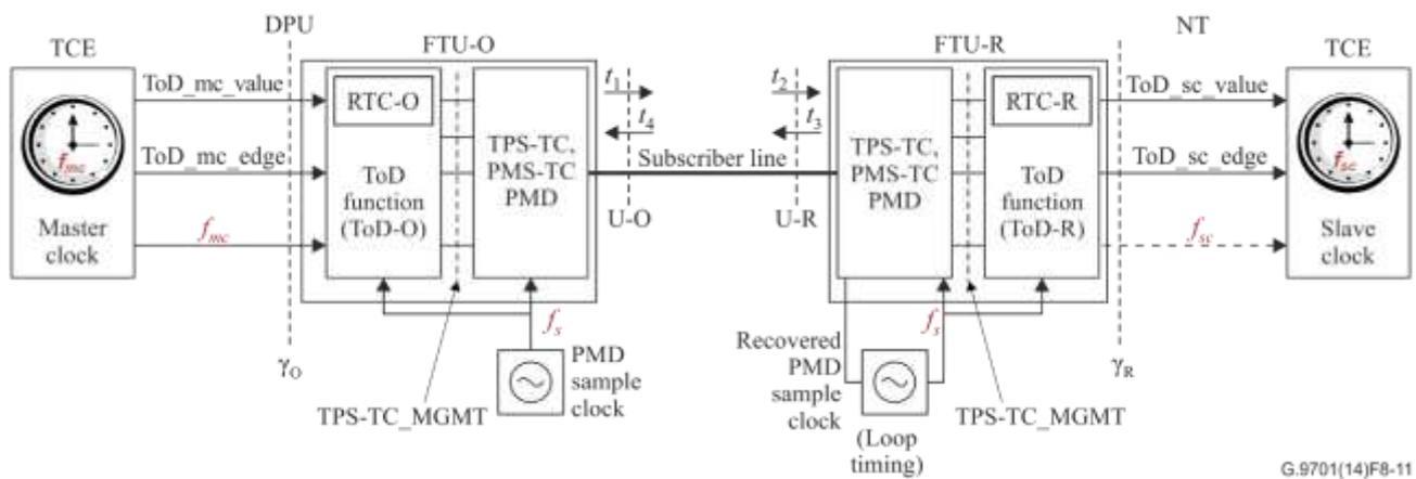
**Figure 8-11 – End-to-end system reference model for time-of-day transport**
