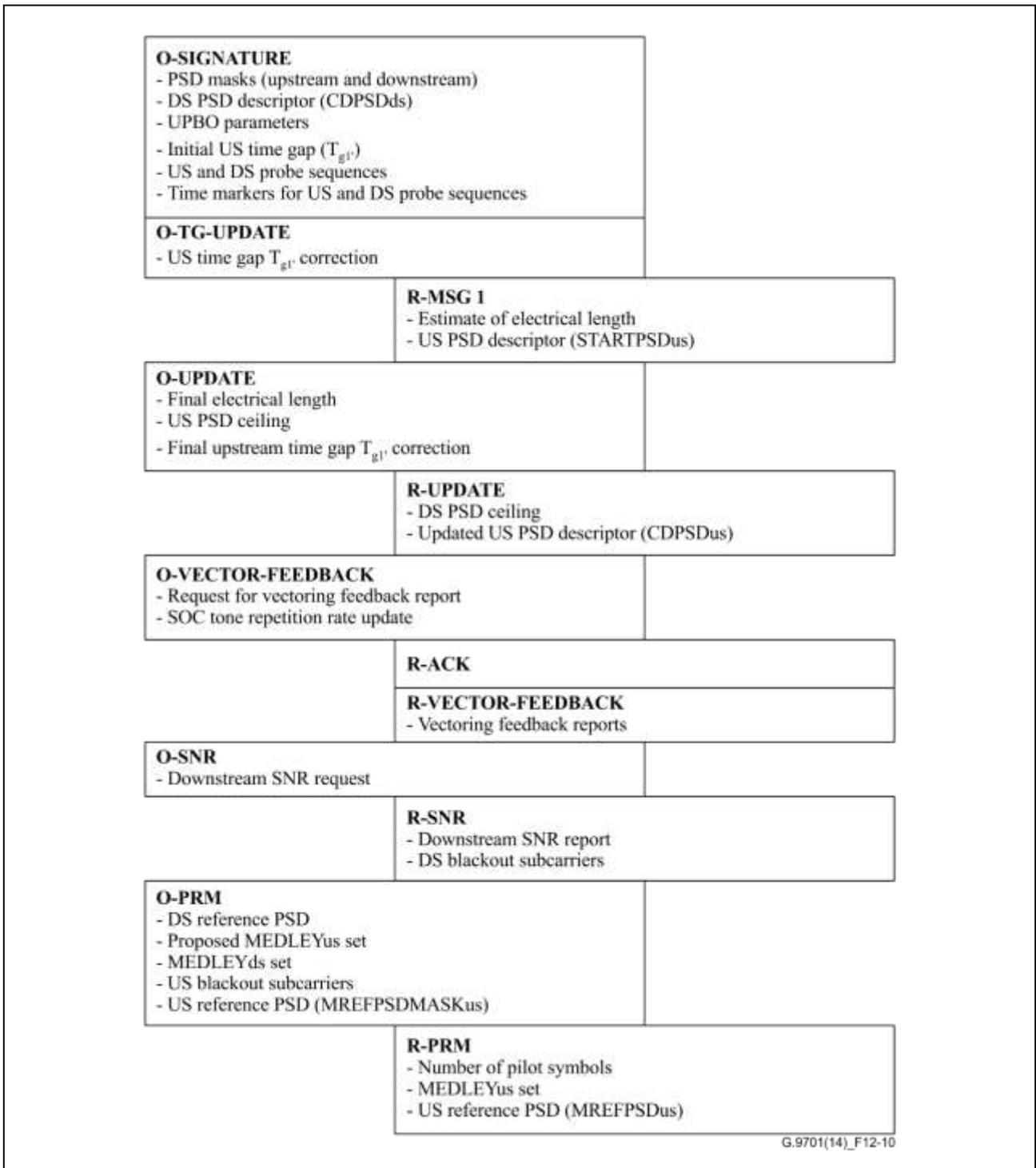
**Figure 12-10 – SOC message exchange during the channel discovery phase**
