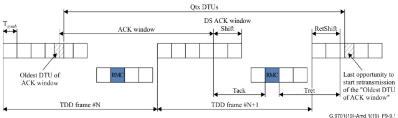
Figure 9-9.1 – Illustration of definition of  $Q_{tx}$
