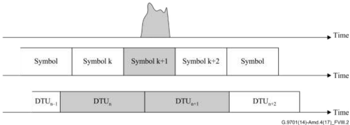
**Figure VIII.2 – An example of DTU corruption due to erasure of a symbol by impulse noise**
