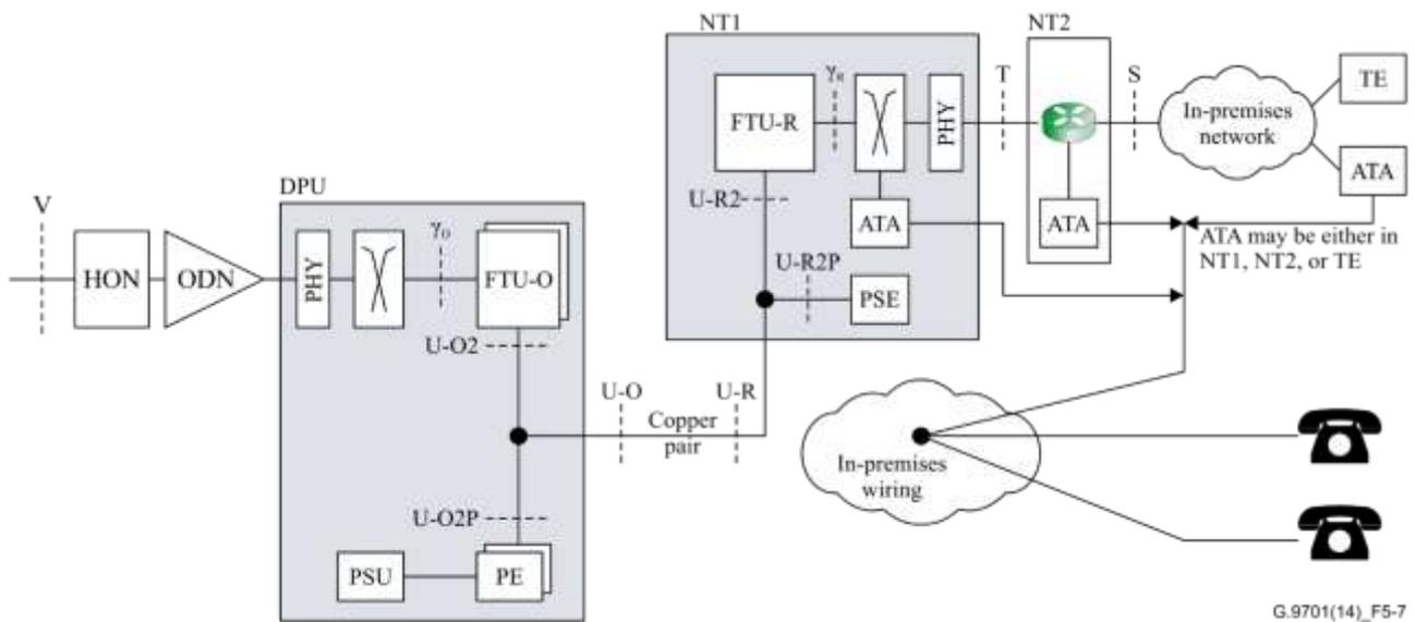
**Figure 5-7 – Application reference model for FTTh with reverse powering and derived POTS not sharing the in-premises wiring with ITU-T G.9701**
