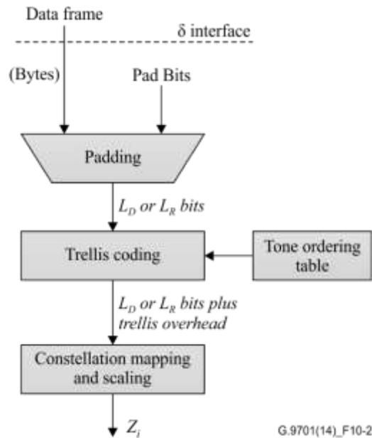
**Figure 10-2 – Functional model of the data symbol encoder**
