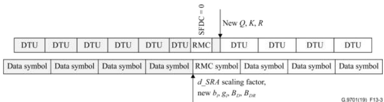
**Figure 13-3 – Timing diagram of SRA transition**
