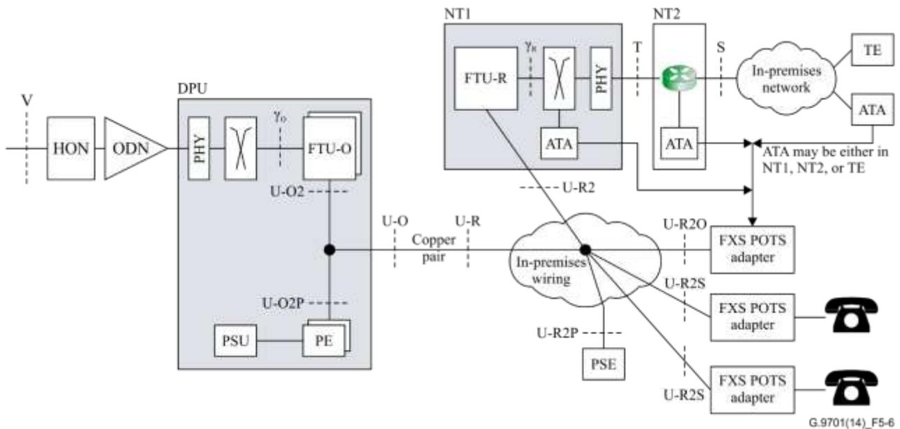
**Figure 5-6 – Application reference model for FTTP with reverse powering and derived POTS**
