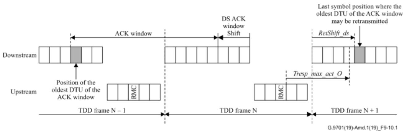
**Figure 9-10.1 – Illustration of parameters  $RetShift$ ,  $T_{resp\_max\_act}$  for the downstream (for  $M_{us} = 5$ ,  $M_{ds} = 8$ ,  $T_{resp\_max\_act\_O} = 6$ ,  $RetShift\_ds = 4$ )**
