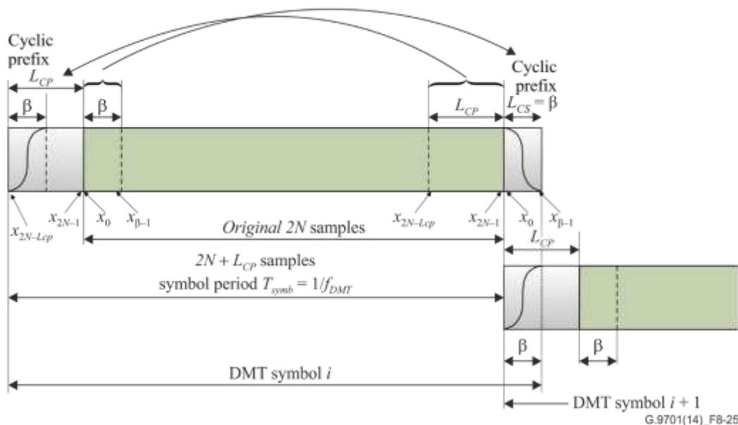
**Figure 10-25 – Cyclic extension, windowing and overlap of symbols**
