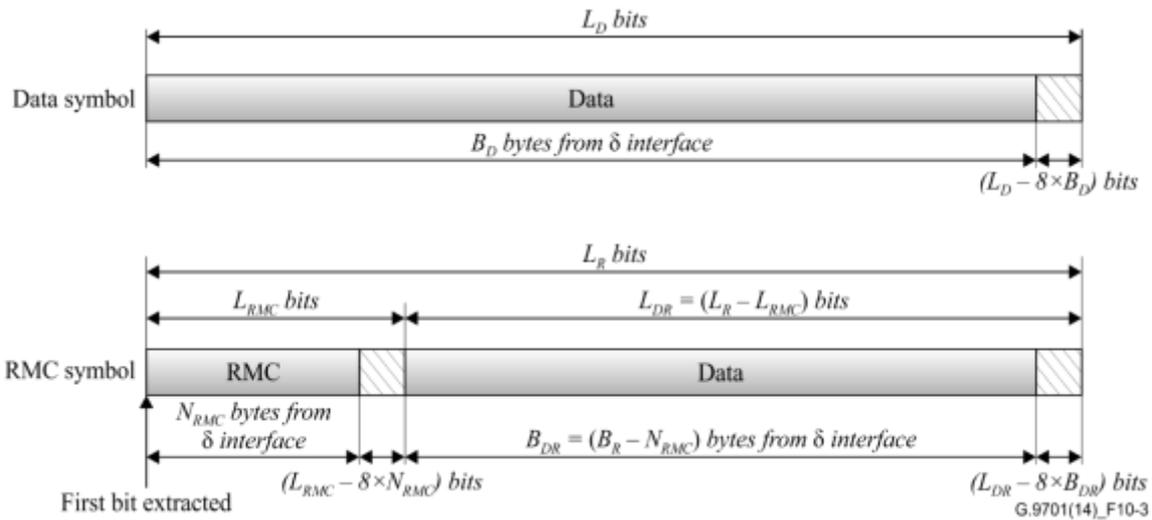
Figure 10-3 – Order of bit extraction from data frame
