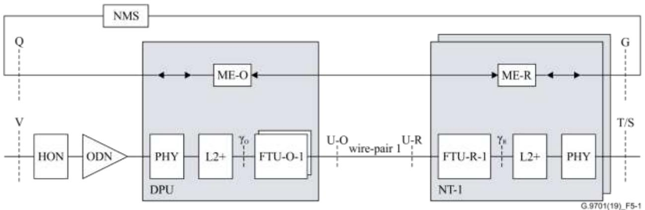
**Figure 5-1 – Reference model of FTTP deployment
