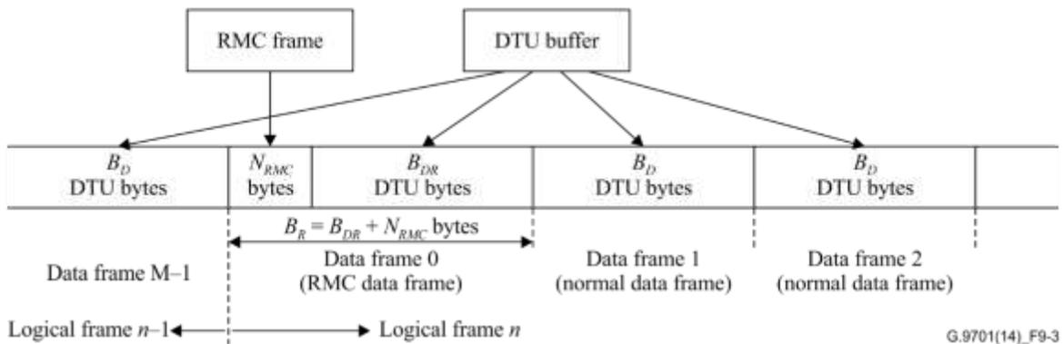
Figure 9-3 – Multiplexing of RMC frame and DTUs into data frames
