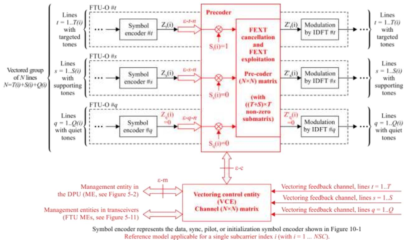
**Figure IV.1 – Vectored group functional model of PMD sub-layer using TGVAds – applicable for a single subcarrier index**
