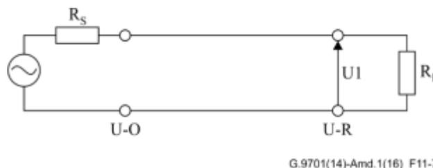
**Figure 11-7 – Voltage across the load without access cabling**
