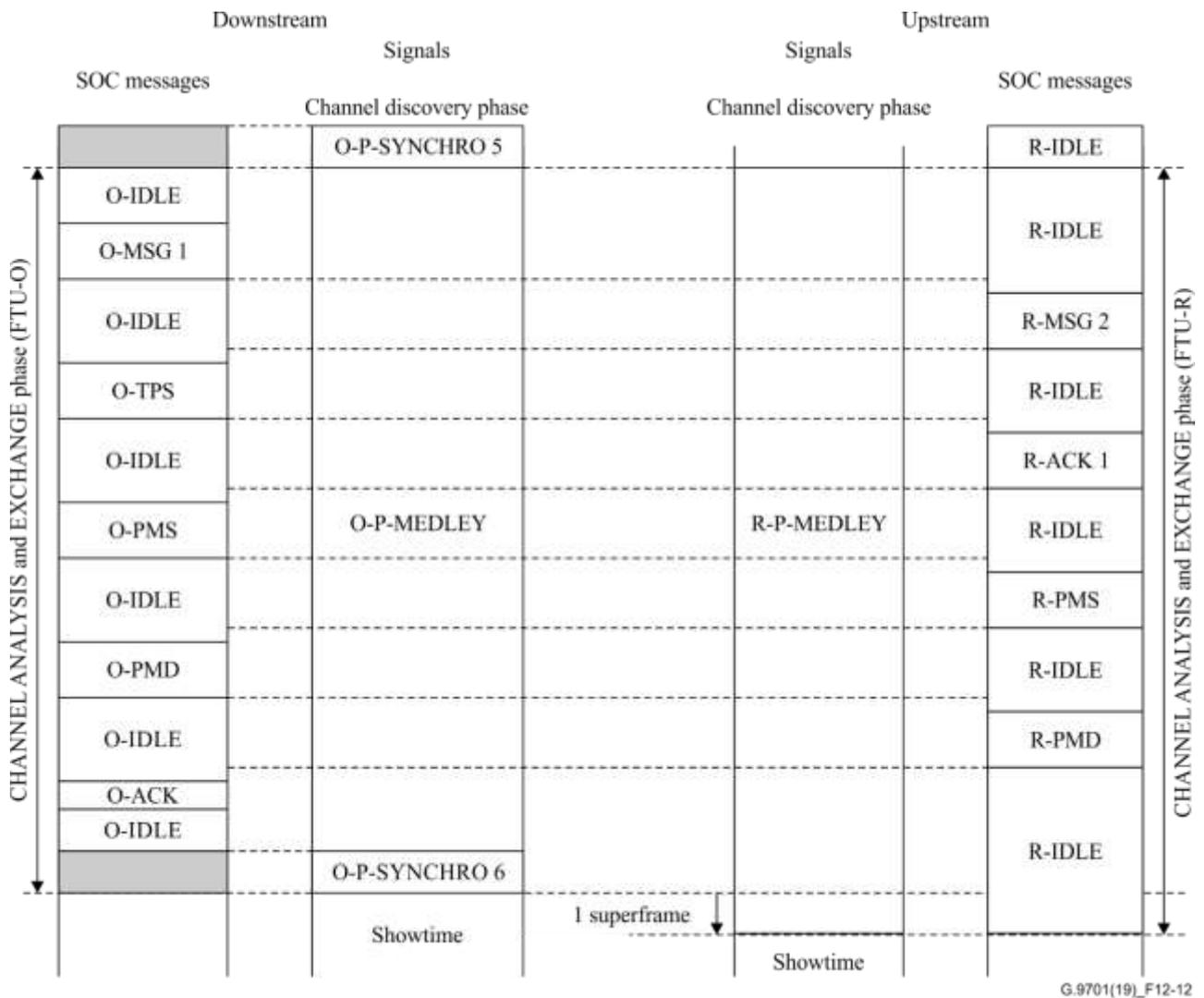
**Figure 12-12 – Timing diagram of the channel analysis and exchange phase**
