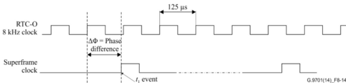
**Figure 8-14 – ToD phase difference ( $\Delta\phi$ ) computation**
