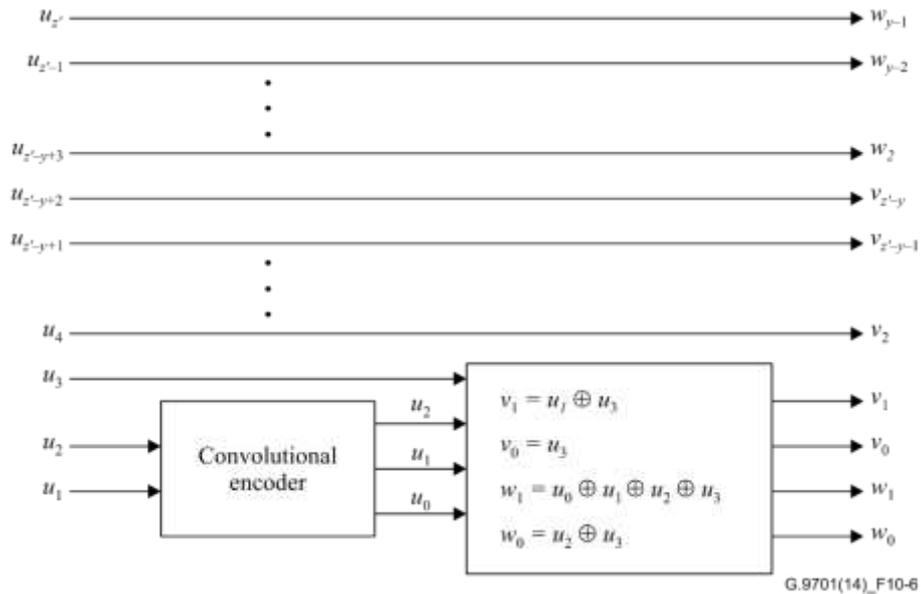
Figure 10-6 – Conversion of  $u$  to  $v$  and  $w$
