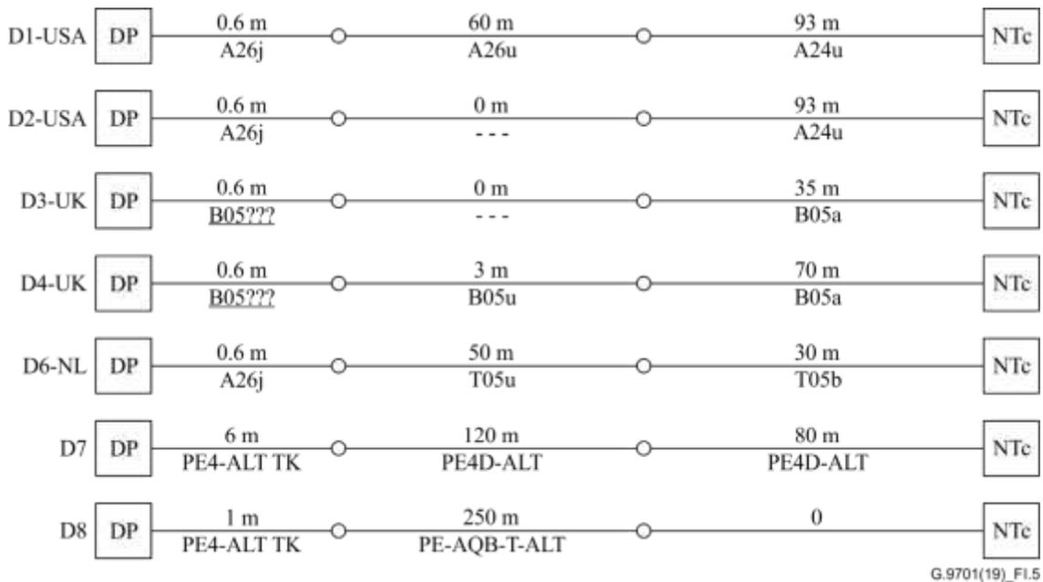
**Figure I.5 – Illustration of final drop loops**
