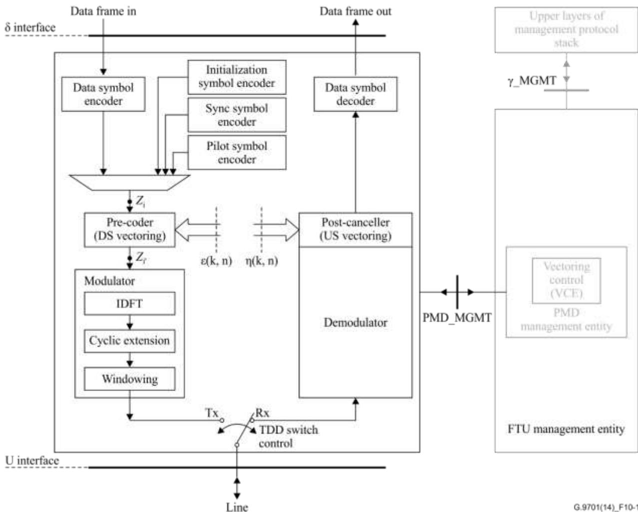
**Figure 10-1 – PMD functional reference model**
