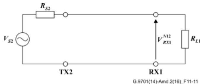
Figure 11-11 – Voltage across the load without access cabling
