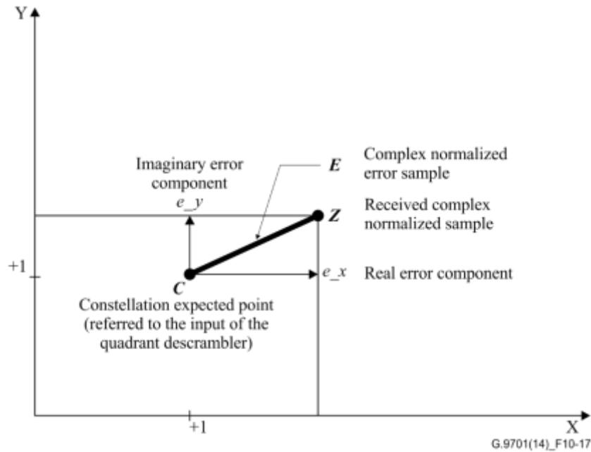
**Figure 10-17 – Definition of the normalized error sample  $E$**
