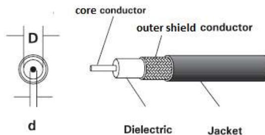
**Figure X.9 – Typical coaxial cable construction [b-Large]**
