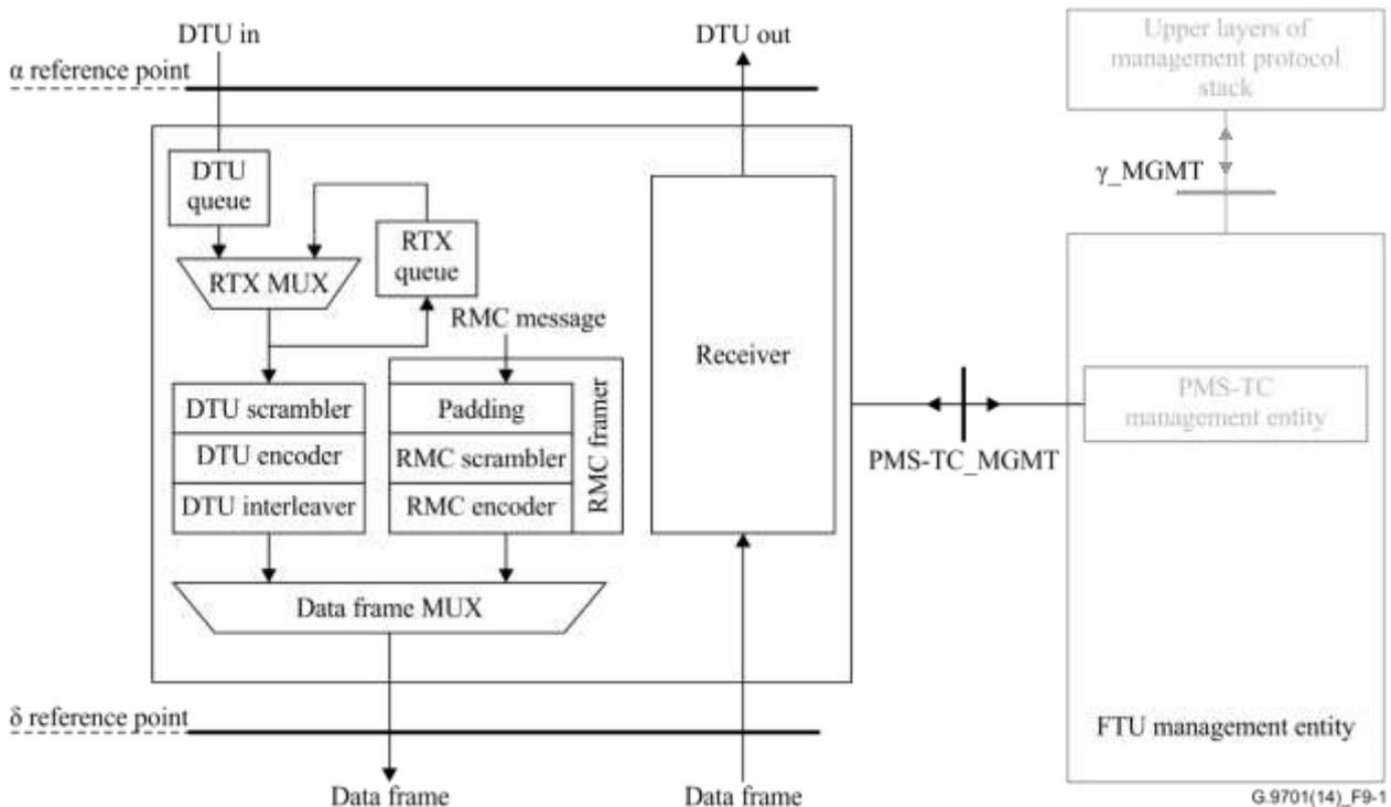
**Figure 9-1 – Functional reference model of PMS-TC**
