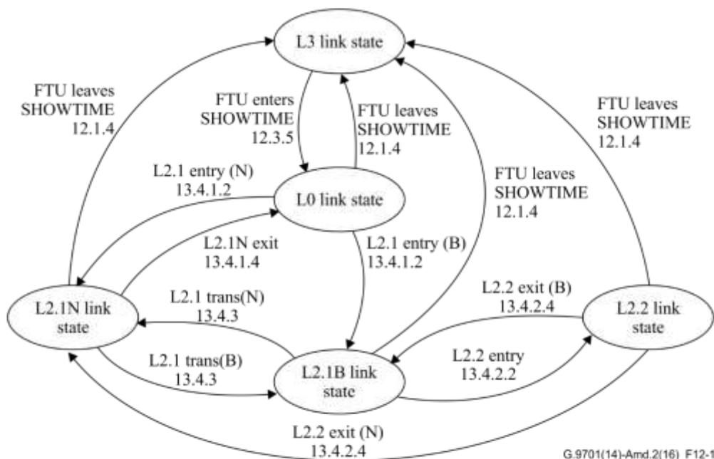
Figure 12-1 – Link states and link-state transition diagram
