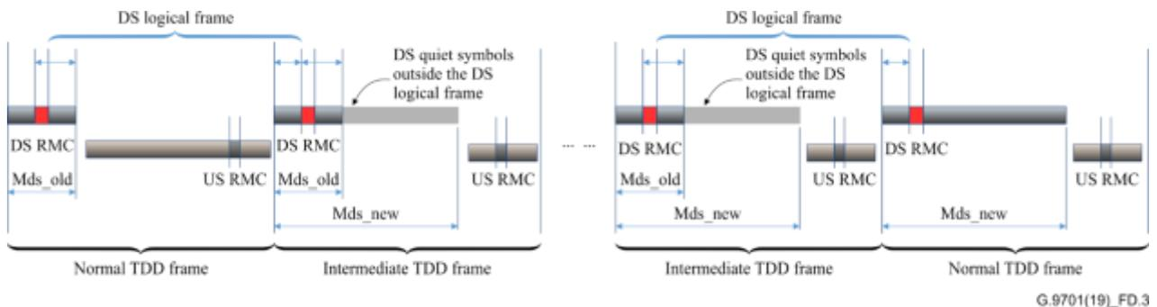
**Figure D.3 – Intermediate TDD frame ( $M_{ds\_new} > M_{ds\_old}$ ) and DS logical frame**
