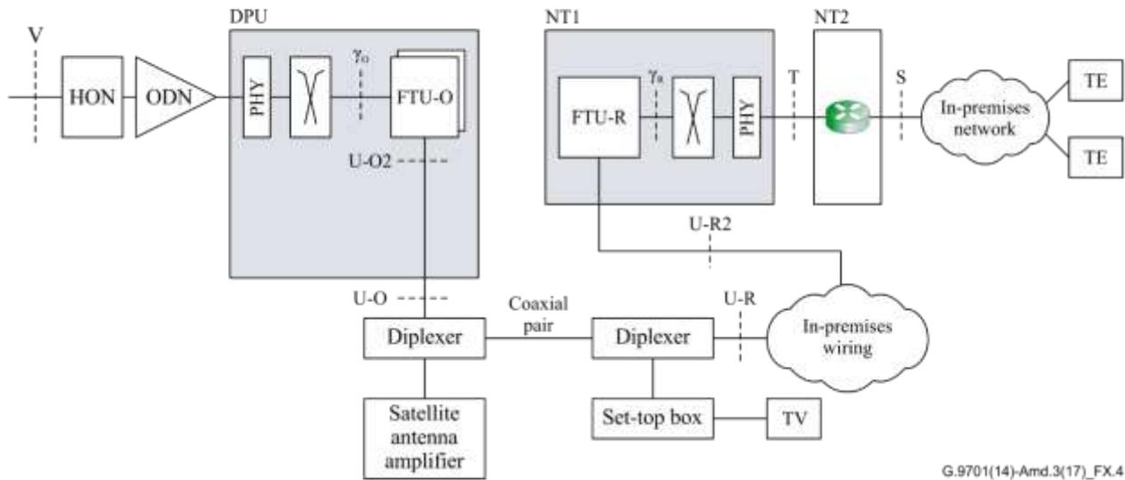
Figure X.4 – Application reference model for coaxial cable medium
