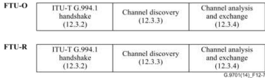
**Figure 12-7 – Timeline of the initialization procedure**
