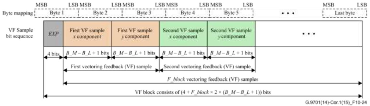
**Figure 10-24 – Format of a VF block**
