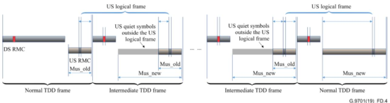
**Figure D.4 – Intermediate TDD frame ( $M_{us\_new} > M_{us\_old}$ ) and US logical frame**
