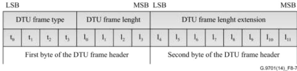
**Figure 8-7 – Format of the DTU frame header**
