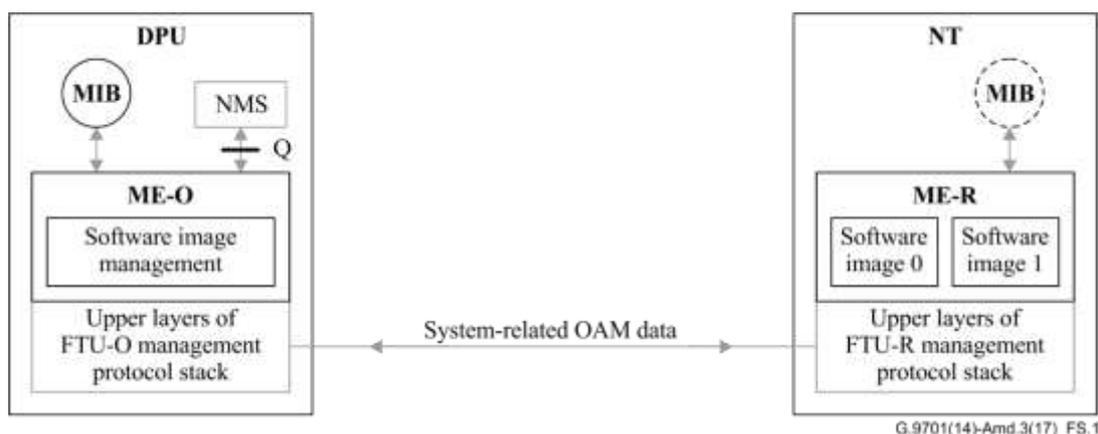
Figure S.1 – Software image management reference model
