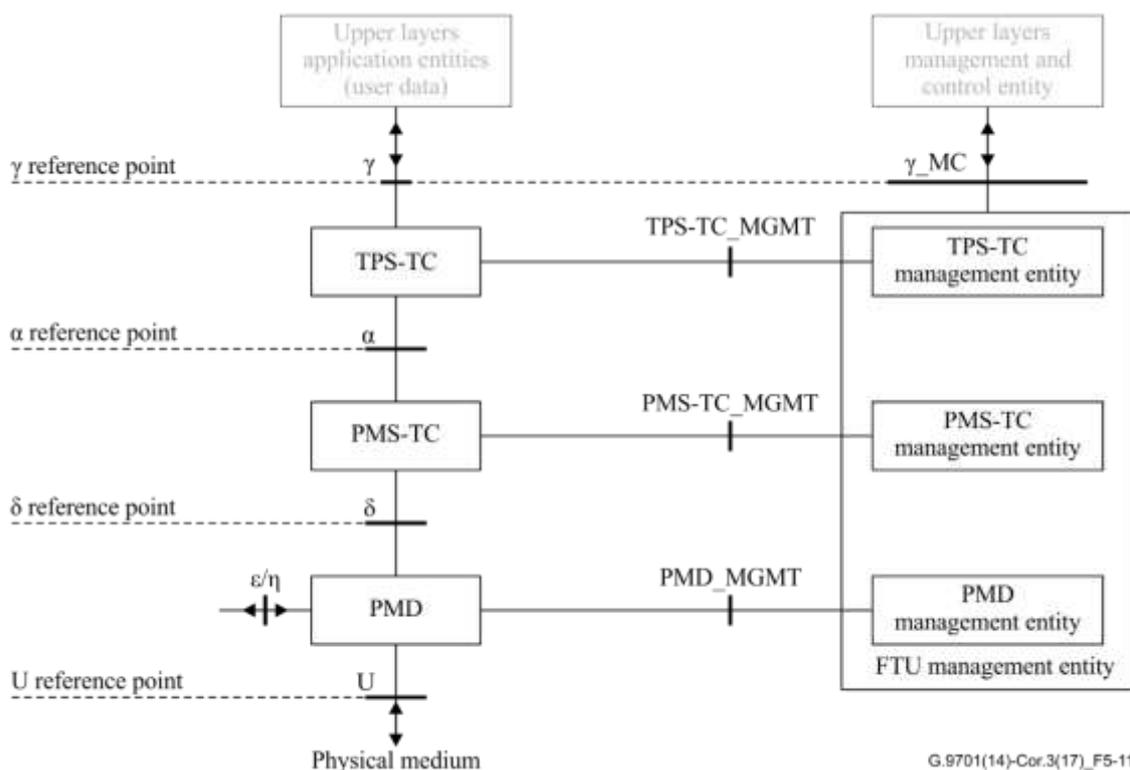
**Figure 5-11 – FTU functional model**
