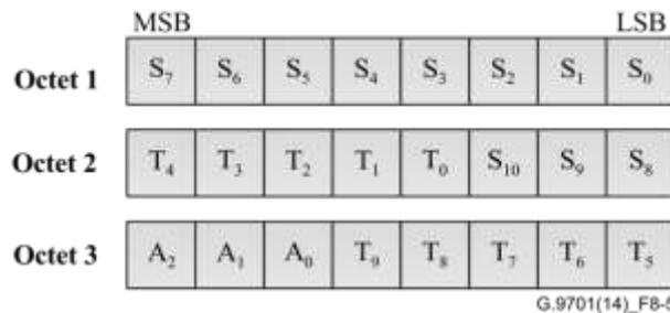
**Figure 8-5 – Bit mapping generic DTU header bytes**
