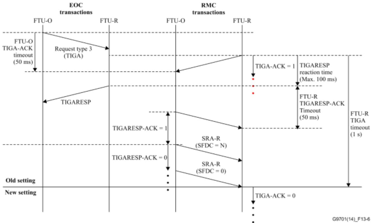
**Figure 13-6 – TIGA procedure with non-segmented messages**
