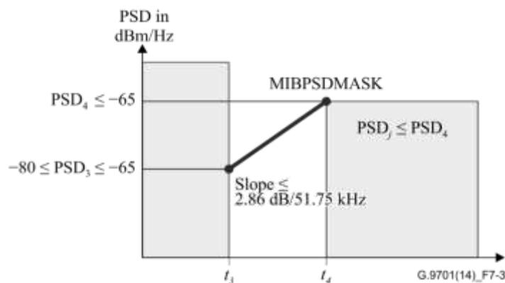
Figure 7-3 – Illustration of the one-slope steep upward shape
