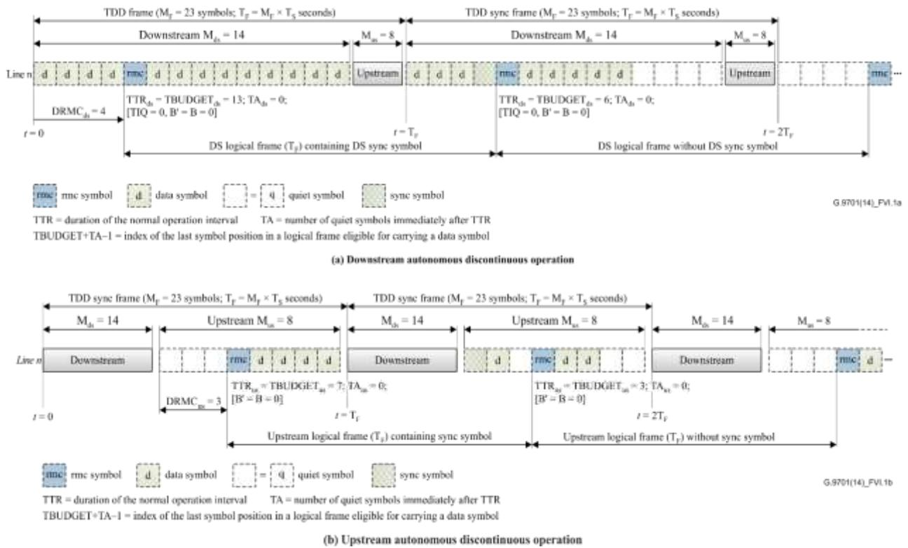
**Figure VI.1 – Discontinuous operation without vectoring
