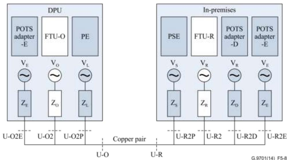
**Figure 5-8 – Electrical reference model for FTUdp with reverse powering and (derived) POTS**
