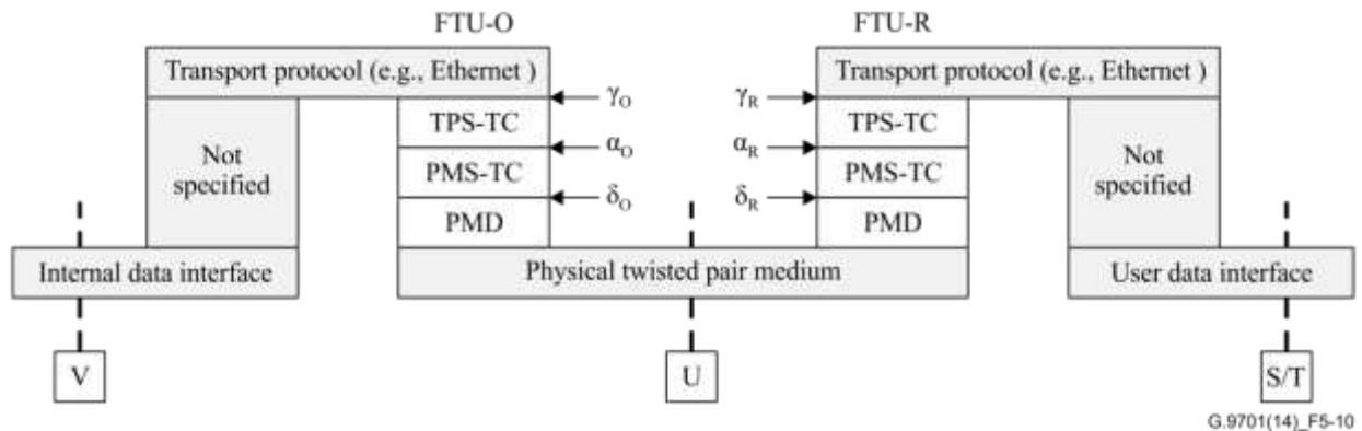
**Figure 5-10 – Data plane protocol reference model**
