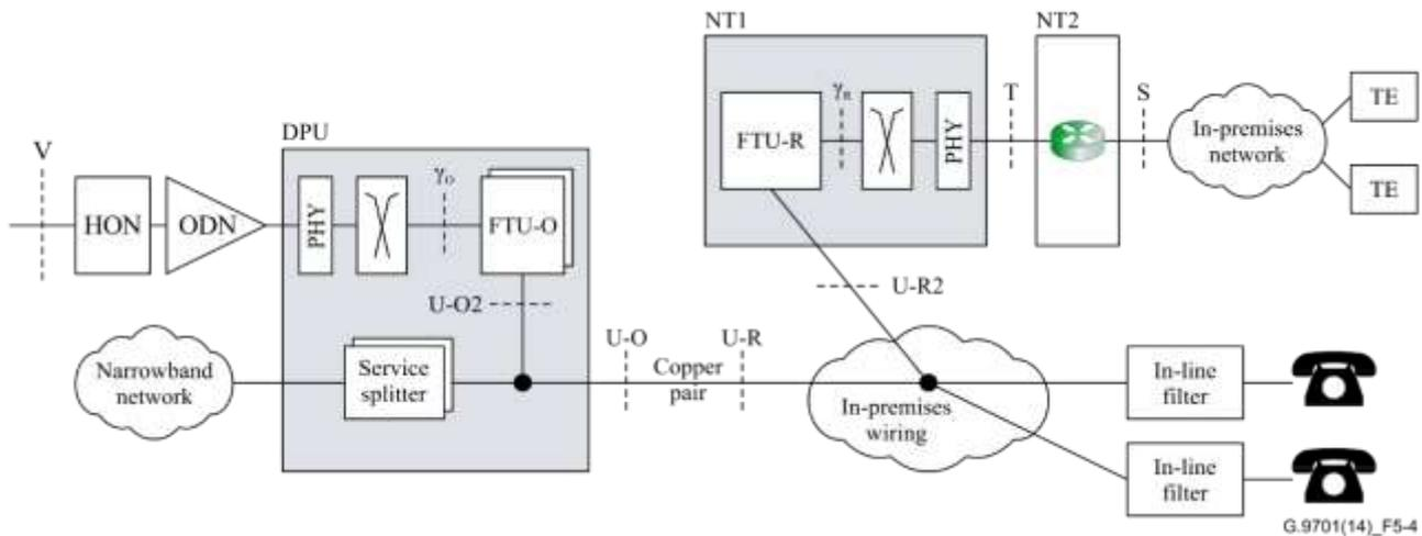
**Figure 5-4 – Application reference model for FTTdp with POTS**
