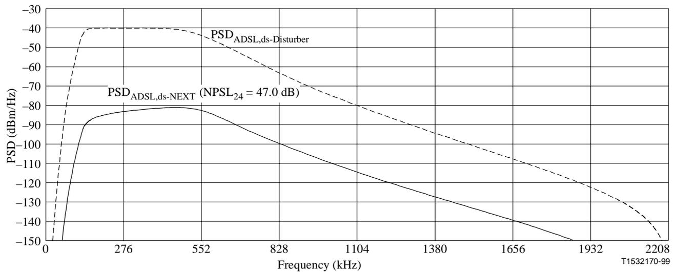
**Figure 34/G.996.1 – 24-disturber G.992.2 (FDM) downstream NEXT**
