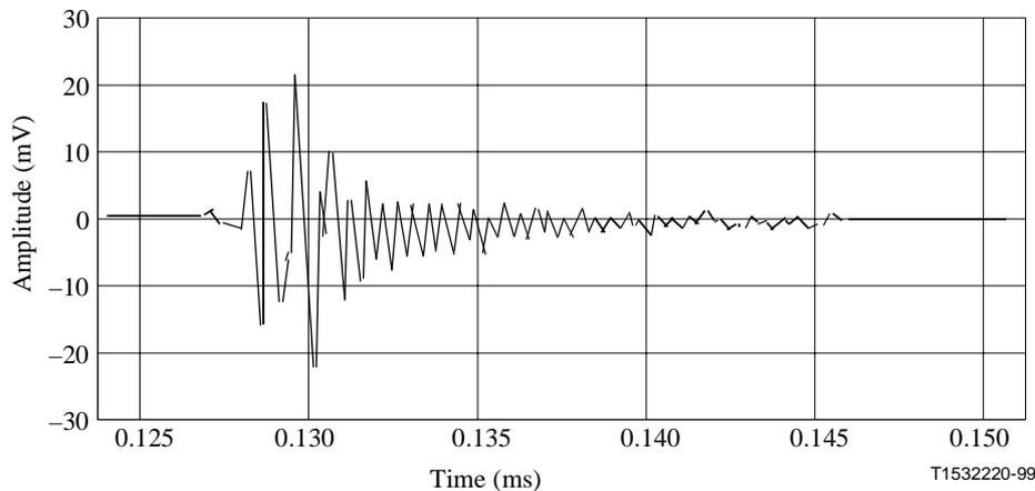
**Figure 39/G.996.1 – Test impulse 1**
