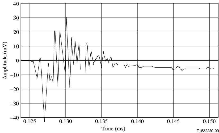
**Figure 40/G.996.1 – Test impulse 2**
