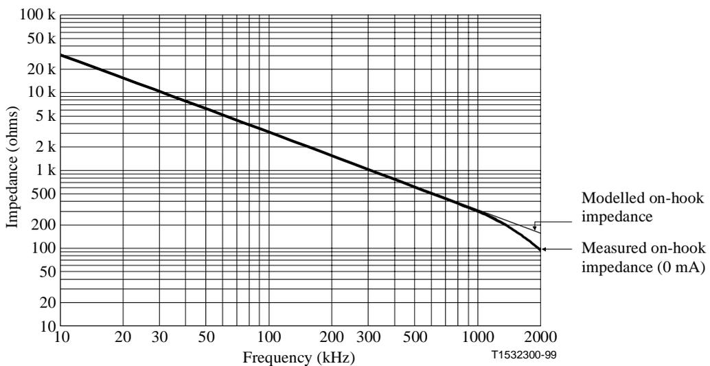
**Figure 47/G.996.1 – Measured and modelled on-hook impedance**
