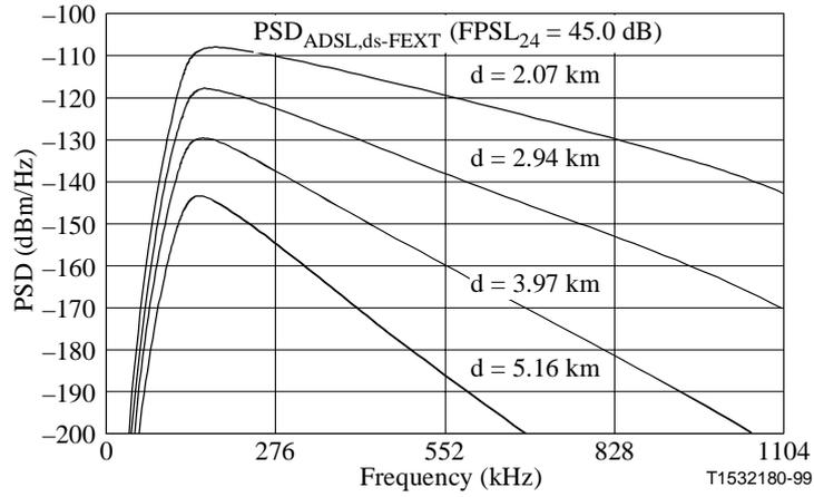
Figure 35/G.996.1 – 24-disturber G.992.1 (FDM) downstream FEXT
