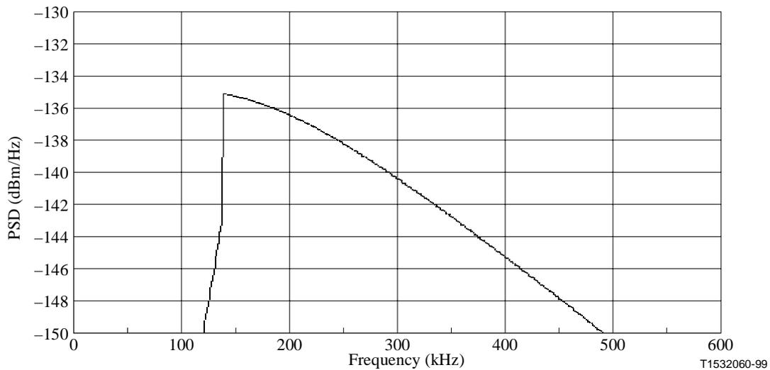
**Figure 23/G.996.1 – 49-disturber downstream G.992.2 FEXT on T loop #7**
