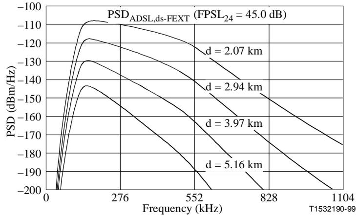
Figure 36/G.996.1 – 24-disturber G.992.2 (FDM) downstream FEXT
