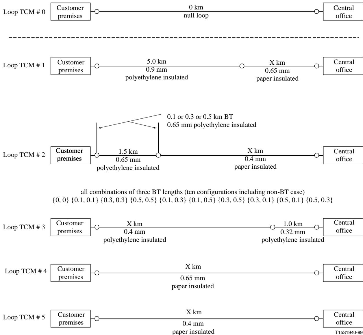
**Figure 11/G.996.1 – Test loop in an environment coexisting with TCM-ISDN DSL**
