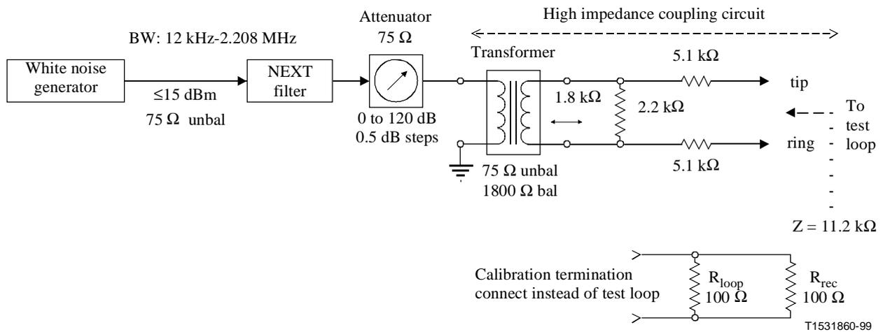
**Figure 3/G.996.1 – High impedance crosstalk injection circuit**
