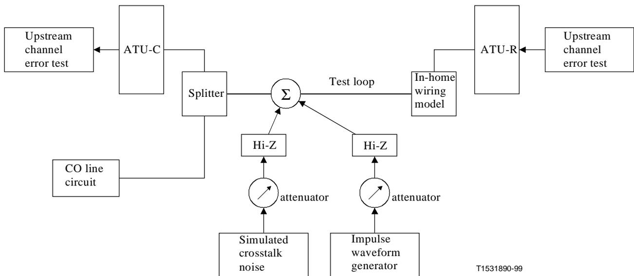
**Figure 6/G.996.1 – Laboratory test set-up for measuring performance margins for the upstream channel without a splitter at the ATU-R**
