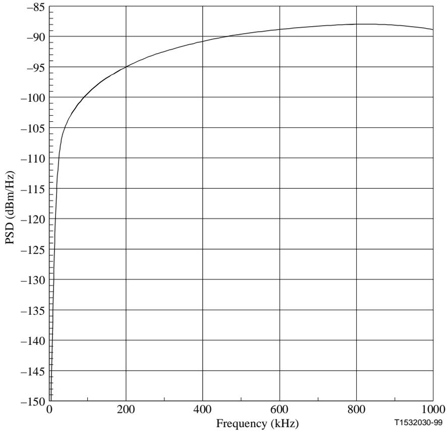
**Figure 20/G.996.1 – 10-disturber downstream G.992.1 NEXT into the upstream**
