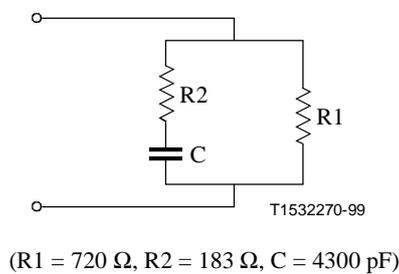
**Figure 44/G.996.1 – Simple model of an off-hook telephone**
