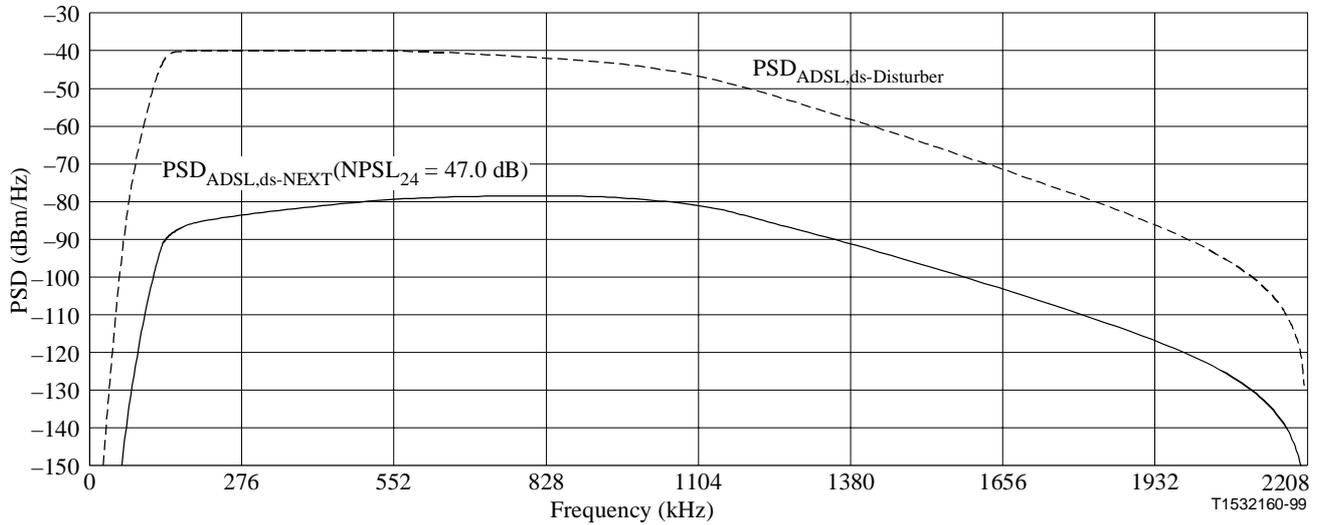
**Figure 33/G.996.1 – 24-disturber G.992.1 (FDM) downstream NEXT**
