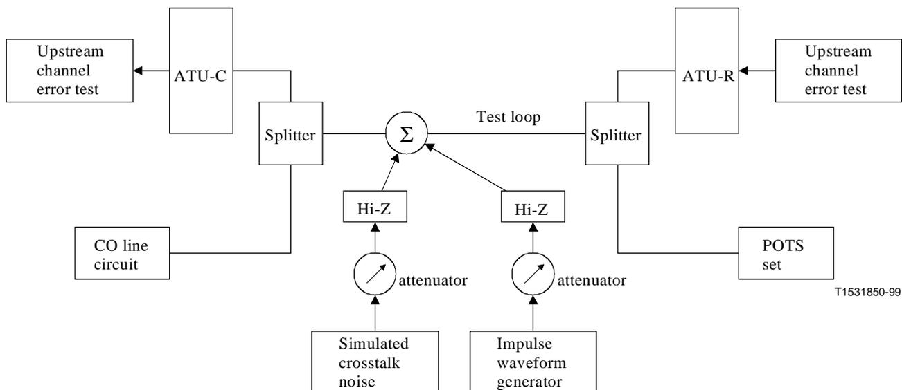
**Figure 2/G.996.1 – Laboratory test set-up for measuring performance margins for the upstream channel with splitters**
