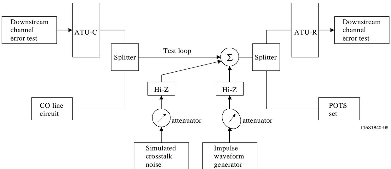
**Figure 1/G.996.1 – Laboratory test set-up for measuring performance margins for the downstream channel with splitters**
