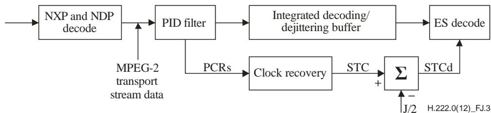
**Figure J.3 – Integrated dejittering and MPEG-2 decoding**
