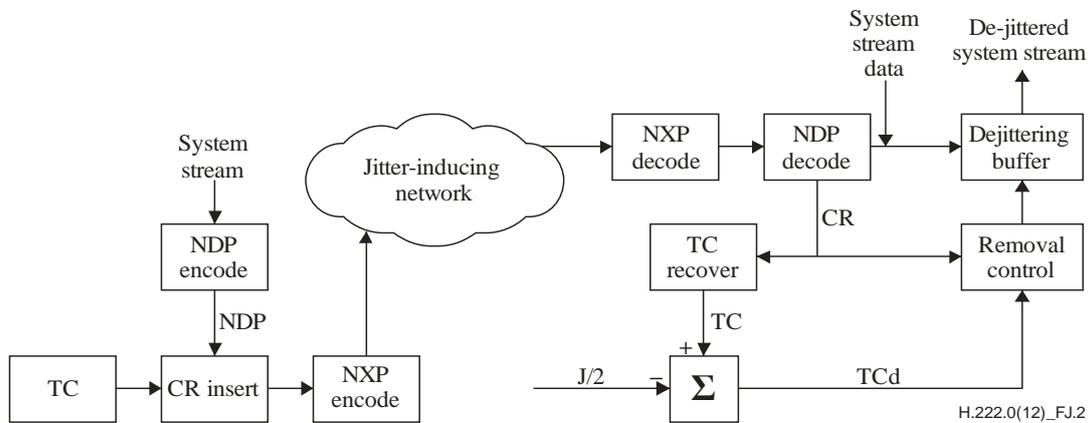
Figure J.2 – Jitter-smoothing using network-layer timestamps
