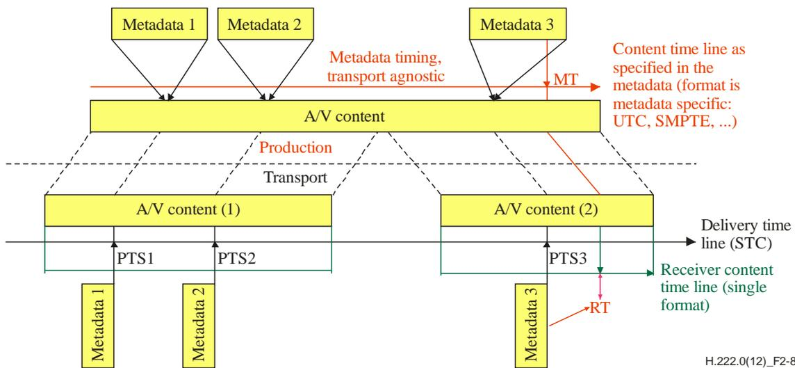
Figure 2-8 – Delivery of metadata in PES packets
