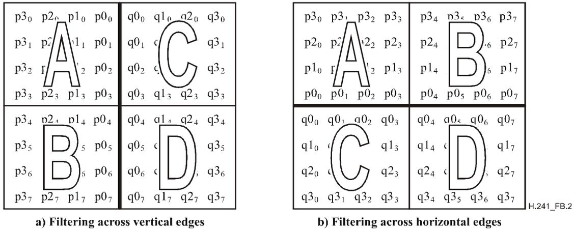
**Figure B.2/H.241 – Arrangement of  $8 \times 8$  blocks when filtering across vertical or horizontal edges**
