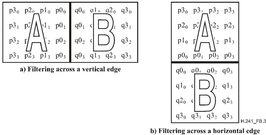
**Figure B.3/H.241 – Arrangement of two  $4 \times 4$  chroma blocks when filtering across a vertical or horizontal edge**
