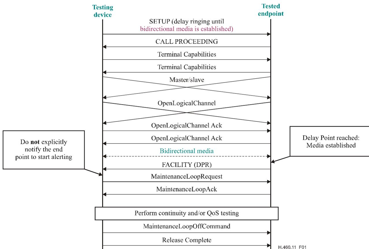
**Figure I.1/H.460.11 – Continuity and/or QoS testing**
