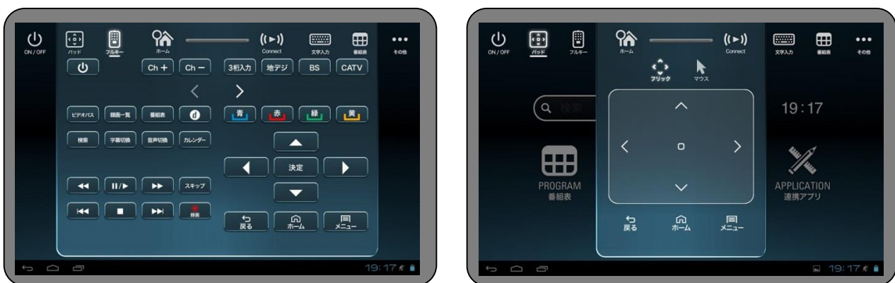
Figure I.1 – Image of tablet remote controller (left: remote controller button emulation, right: mouse emulation)
