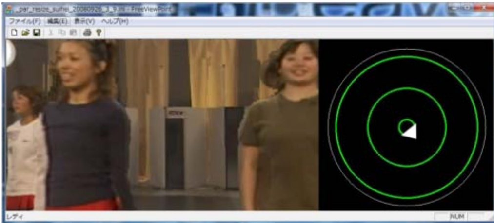
Figure I.5 – Example of walk-through view generation in the second layer of multilayer multi-view video plus depth
