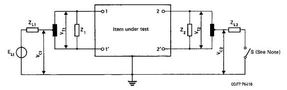
*Note* – Measurements are normally made, and limits specified, with switch S closed. However, for certain equipments, e.g. those described, in Recommendation Q.45, it may be necessary to specify limits for longitudinal conversion transfer loss (LCTL) with switch S closed and with switch S open.
