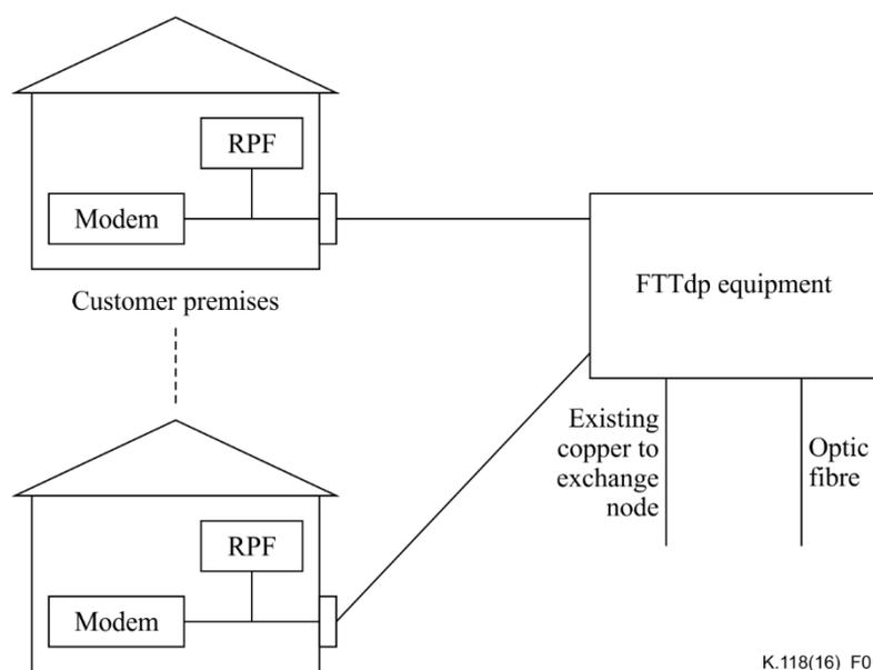
In some implementations the FTTdp equipment may be connected to the existing copper cable from the exchange node until all customers are converted to VoIP.
