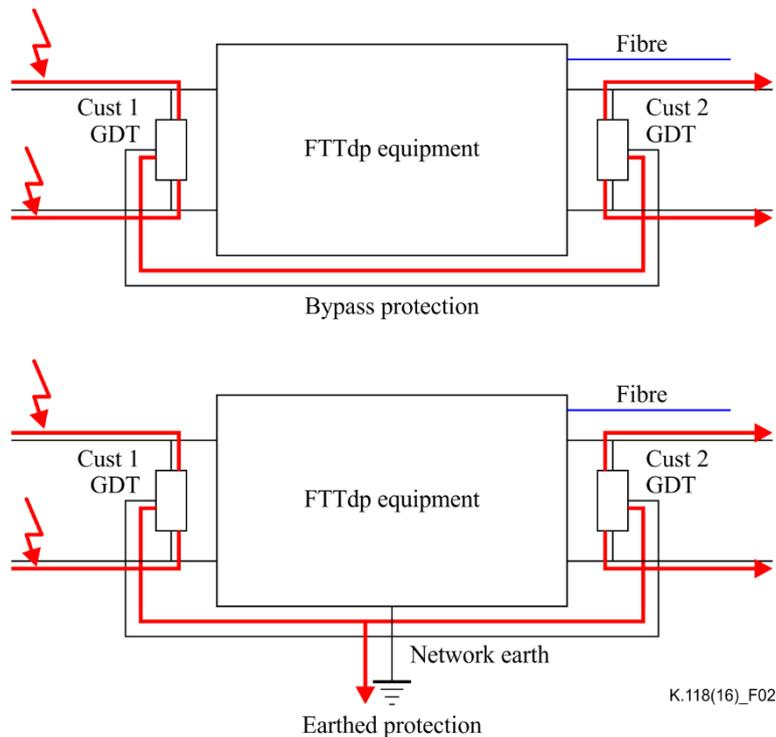
**Figure 2 – Pictorial illustration of bypass and earthed protection**
