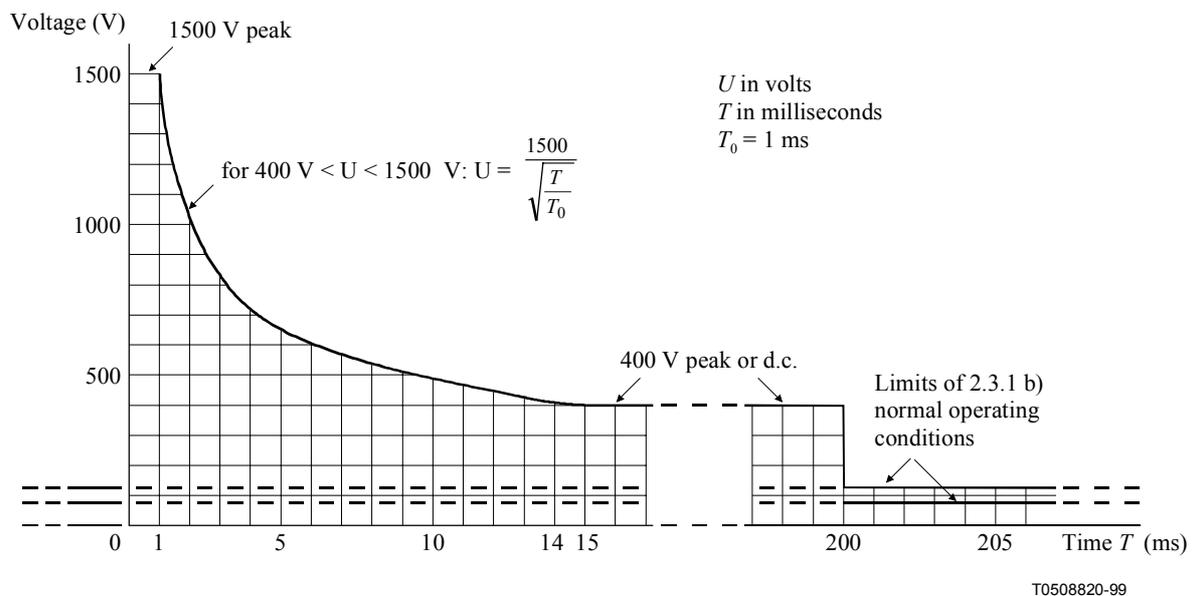
**Figure A.1/K.50 – Maximum voltages permitted after a single fault**
