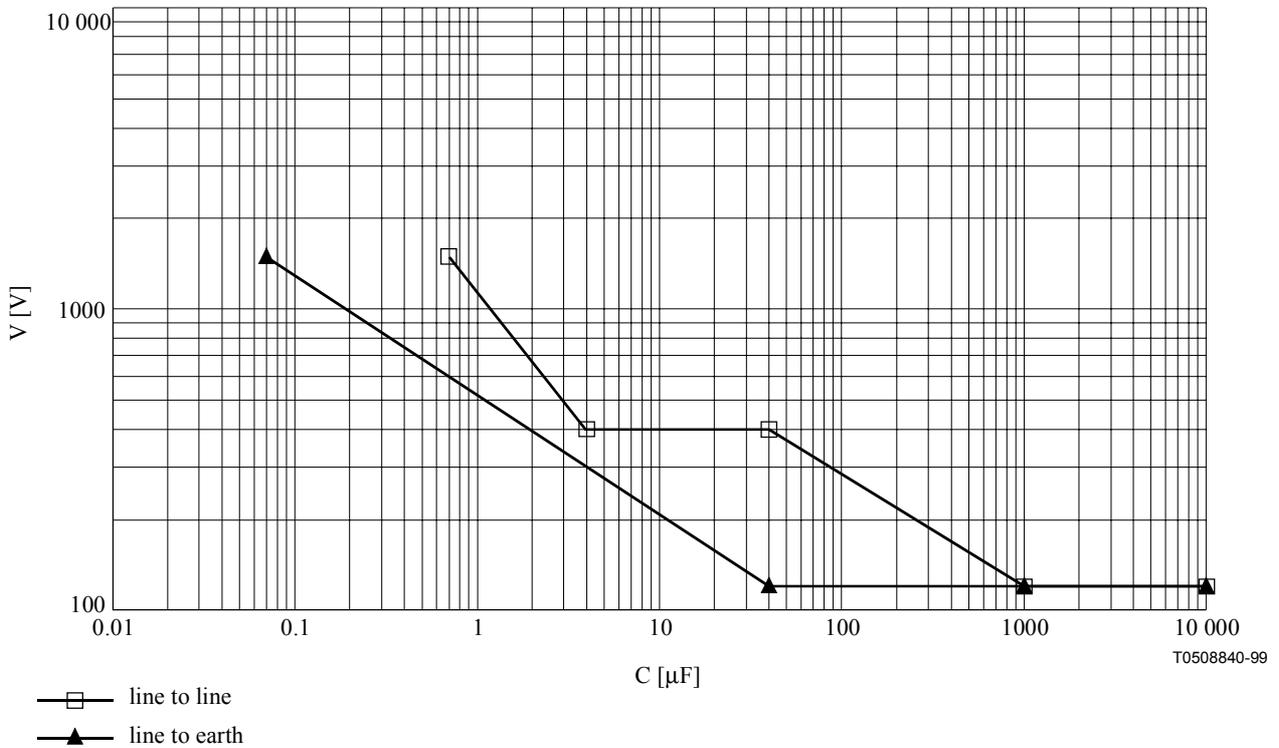
**Figure B.2/K.50 – Limits for capacitance values of RFT circuits or the total system**
