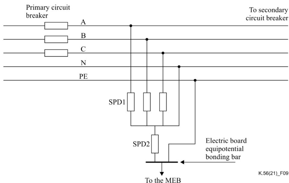
**Figure 9 – Schemes for SPD installation on TN-S, TT or IT power systems**
