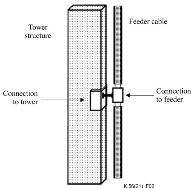
**Figure 2 – Example of installation of earthing kit on feeder cable (protective coating not shown)**
