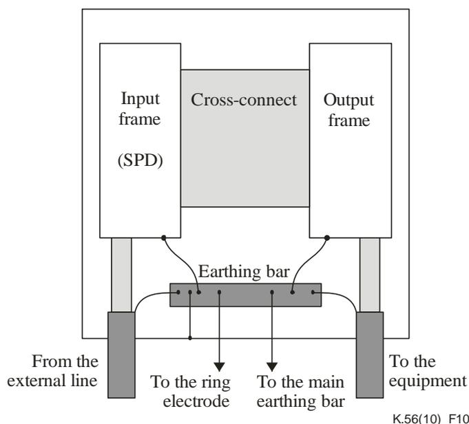
**Figure 10 – Diagram of the telecommunication distribution frame**
