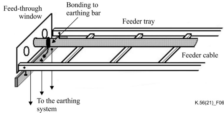
**Figure 6 – Example of earthing the feeder cable at the feed-through window**
