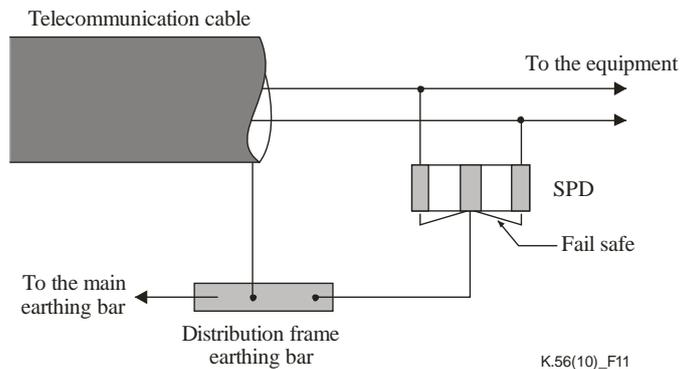
**Figure 11 – Installation of SPD in the distribution frame**
