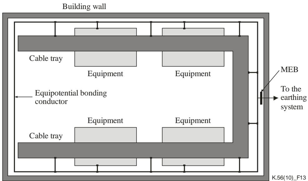
**Figure 13 – Equipotential bonding conductor around the equipment room**
