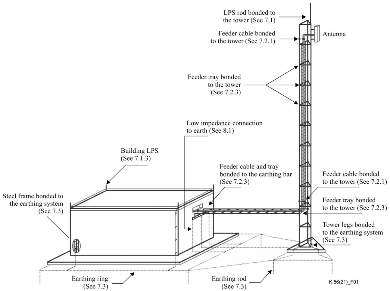
**Figure 1 – General view of earthing and bonding procedures in the external area**
