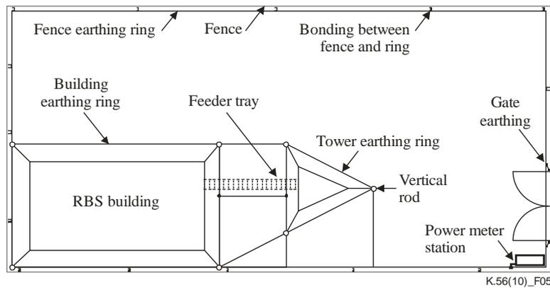
**Figure 5 – Earthing system of the RBS**
