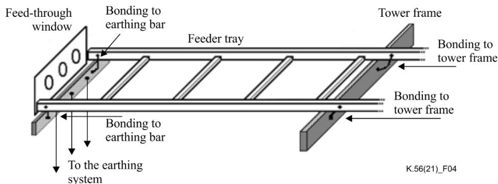
**Figure 4 – Feeder tray bonded at both ends**
