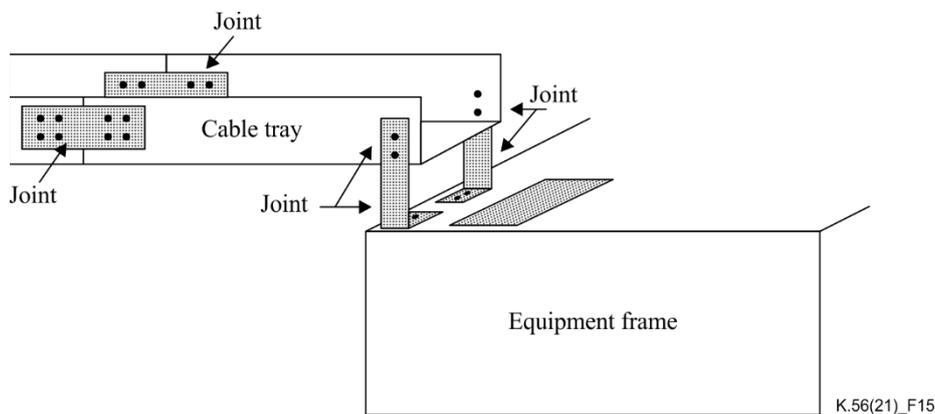
**Figure 15 – Detail of the electrical continuity in trays and equipment frame**
