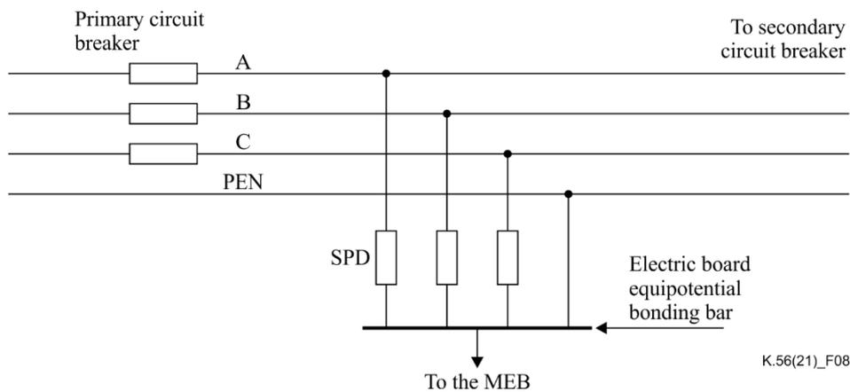
**Figure 8 – Scheme for SPD installation on TN-C power systems**
