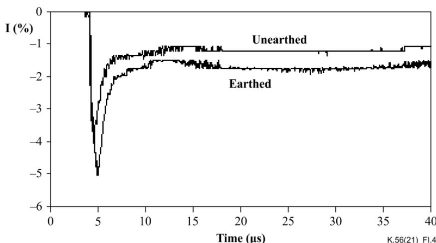
**Figure I.4 – Feeder current as a function of the bonding procedure at ground level**
