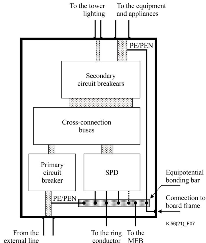
**Figure 7 – Diagram of the electric board**
