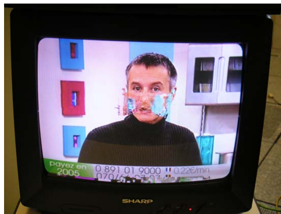
Figure I.2 – Example of the impact of impulse noise on the TV service
