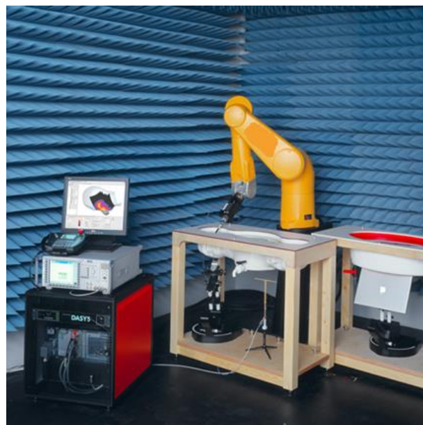
Figure 6-3 – A head SAR measurement system where phantom, robot with calibrated probe, and a post-processing unit is shown
